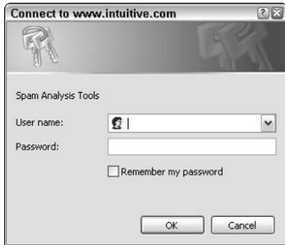
Figure 14-1: The .htaccess file forces visitors to log in before viewing the directory.
