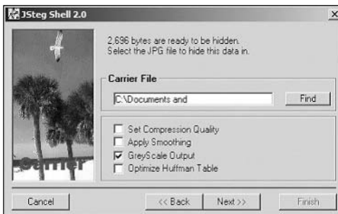
Figure 15-18: Jsteg screen for picking the over file you want to hide data within
