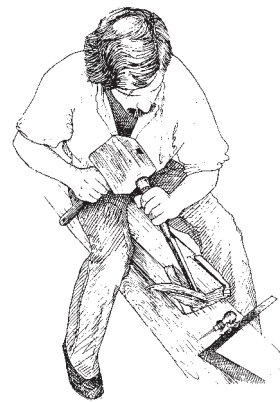
A framing chisel is stout enough to work as a wedge...
