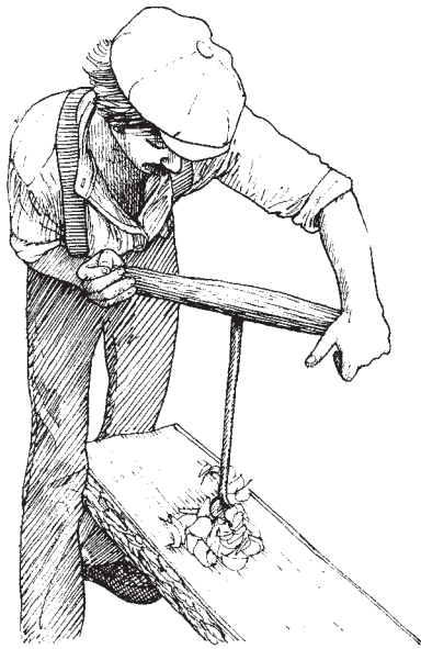
The screw-pointed, spiral auger draws itself into the wood.
