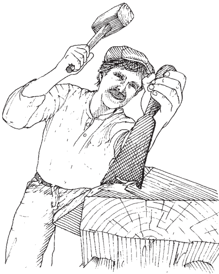
The old fermoir chisel had a double-beveled edge.
