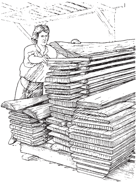
Sawn and separated by stickers, the boards dry under cover for a few years.
