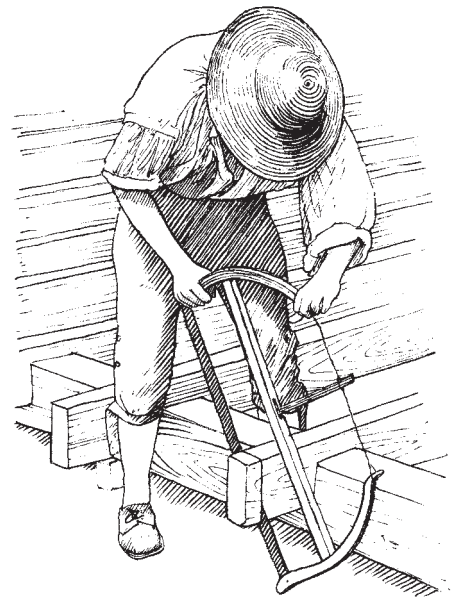
Ease the tension on your bucksaw frame when you're done for the day.
