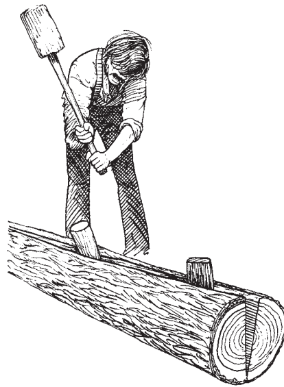
LEFT: The beveled striking head keeps the glut from splintering.
