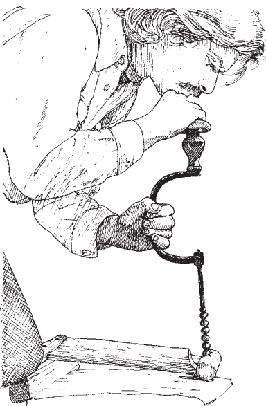
A brace and bit makes the boring continuous.
