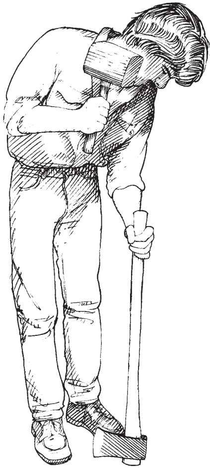
Drive the helve into the eye as inertia holds the head.
