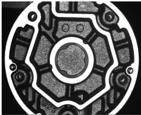
FIGURE 3.27 Images taken under directional field illumination.
