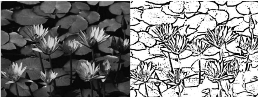
FIGURE 2.17 Sample image and its threshold version.
