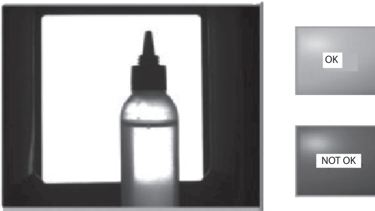
FIGURE 4.12 Profile inspection—checking bottle fill levels.
