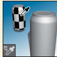
The 3D Material Eyedropper tool loads selected material from a 3D object.
