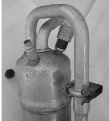
Figure 3.135 Ford A/C compressor cycling switch (integrated into the accumulator/low pressure service port)
