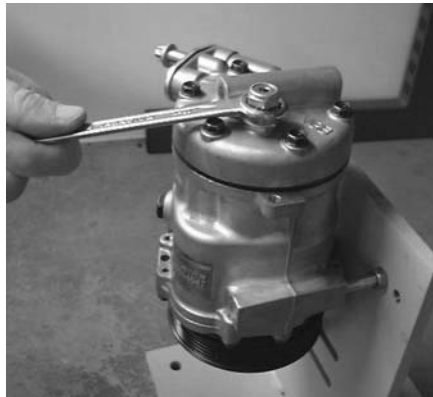
Figure 5.57 Removal of high pressure relief valve
