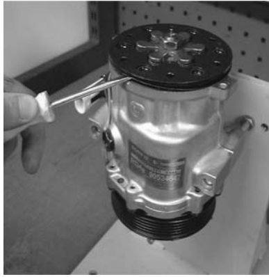
Figure 5.53 Removal of valve plate
