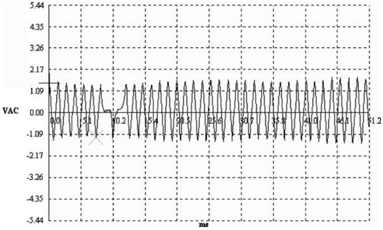
Figure 3.110 AC PWM waveform produced by an inductive speed sensor with a missing tooth on the rotor
