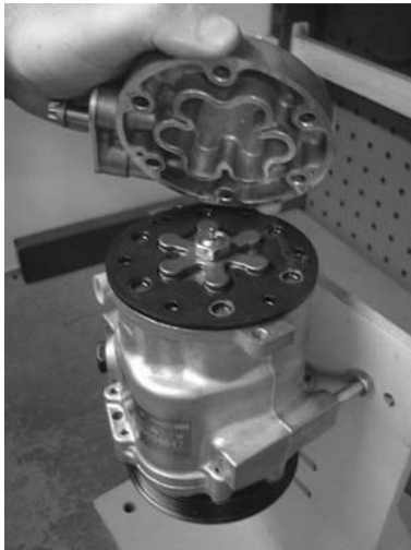
Figure 5.52 Removal of cylinder head
