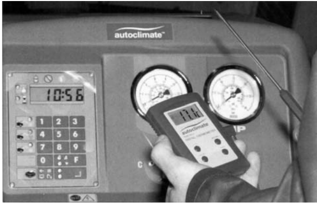
Figure 5.11 Ambient temperature check
