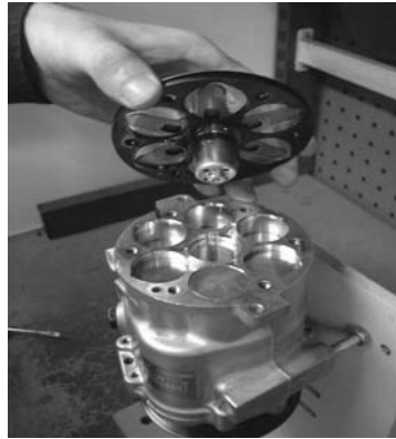
Figure 5.54 Valve plate removed showing MFCV
