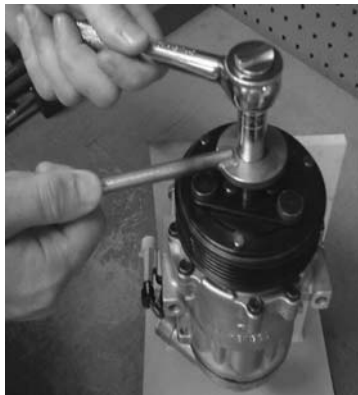
Figure 5.33 Removal of armature retaining nut
