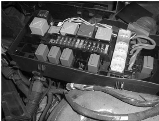
Figure 3.139 Ford BJB contains A/C switch and WOT relay
