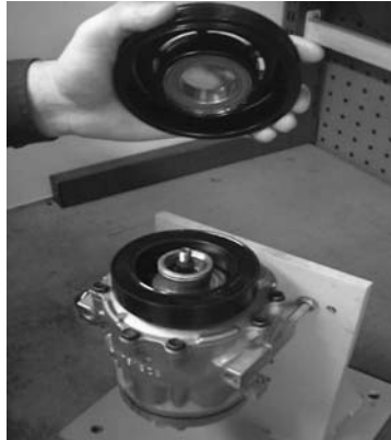
Figure 5.37 Remove rotor (note – bearing staked into place)
