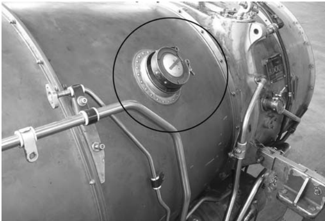
Figure 1.60 Gas turbine engine showing the outlet feed to the A/C system (courtesy of RAF Coltishall)
