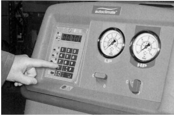
Figure 5.22 Charging with refrigerant
