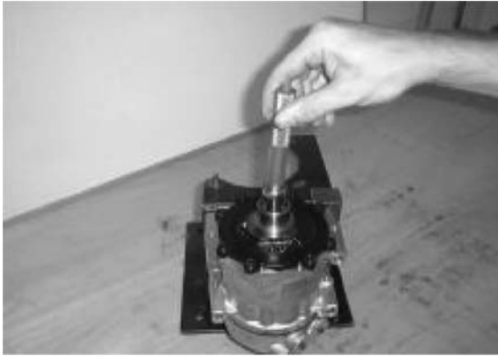
Figure 5.50 Replacement of lip seal
