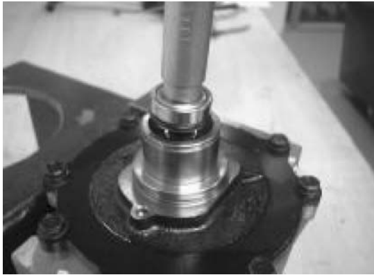
Figure 5.48 Shaft seal removal
