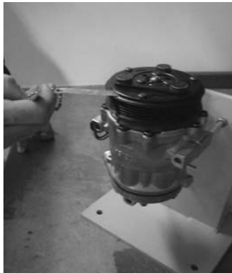
Figure 5.45 Check air gap with feeler gauges
