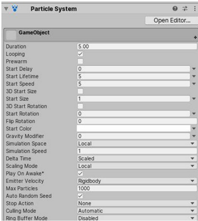
Figure 3-26. The first settings in a Particle System component
