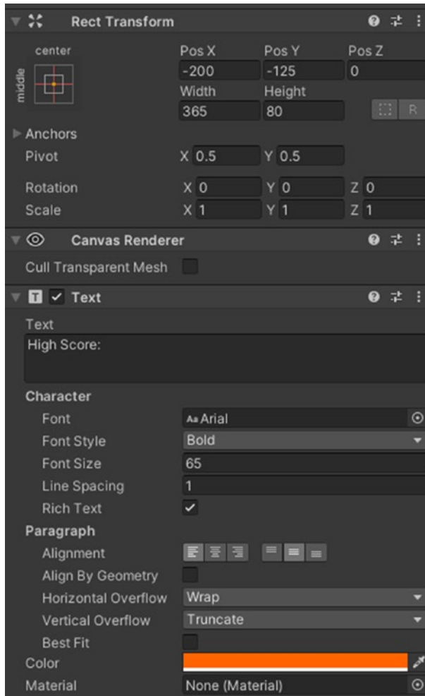
Figure 6-27. The Rect Transform and Text components of HighScoreLabel
