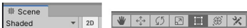
Figures 4-1 and 4-2. The 2D view button (left) and the Rect tool (right)
