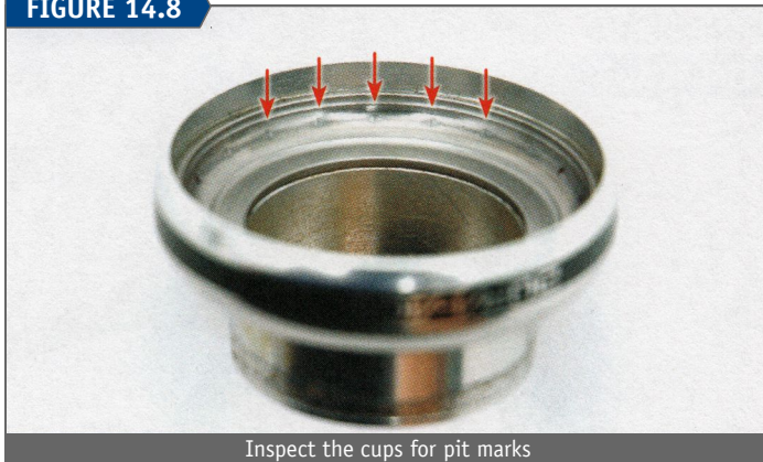
Inspect the cups for pit marks
