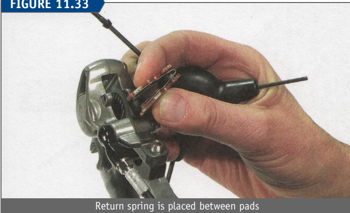
Return spring is placed between pads
