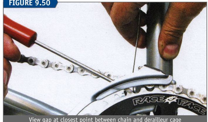
View gap at closest point between chain and derailleur cage
