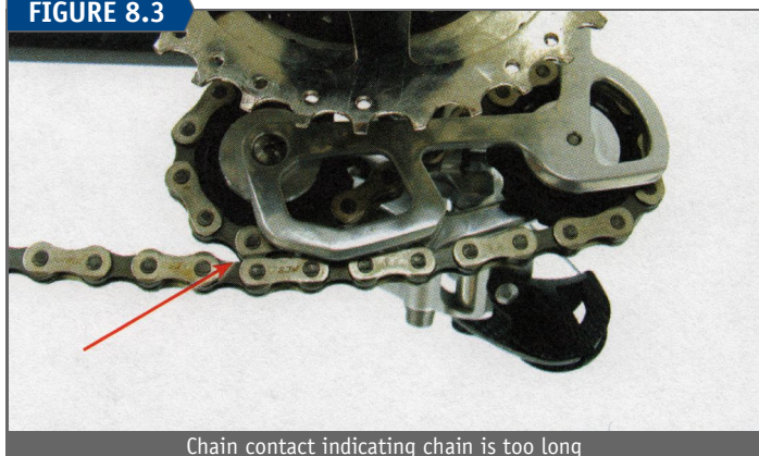
Chain contact indicating chain is too long
