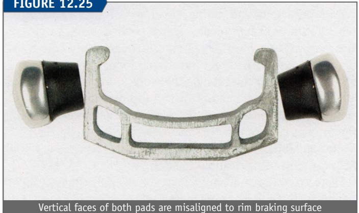
Vertical faces of both pads are misaligned to rim braking surface
