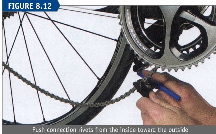
Push connection rivets from the inside toward the outside
