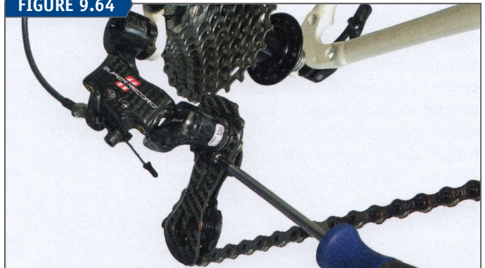
Adjusting the Campagnolo® B-screw at the cage pivot
