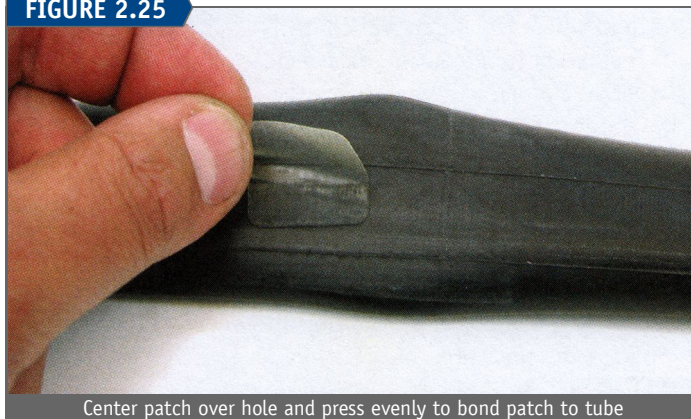
Center patch over hole and press evenly to bond patch to tube
