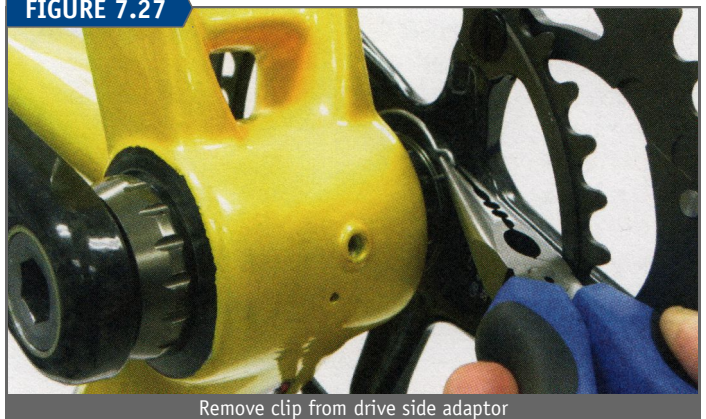
Remove clip from drive side adaptor
