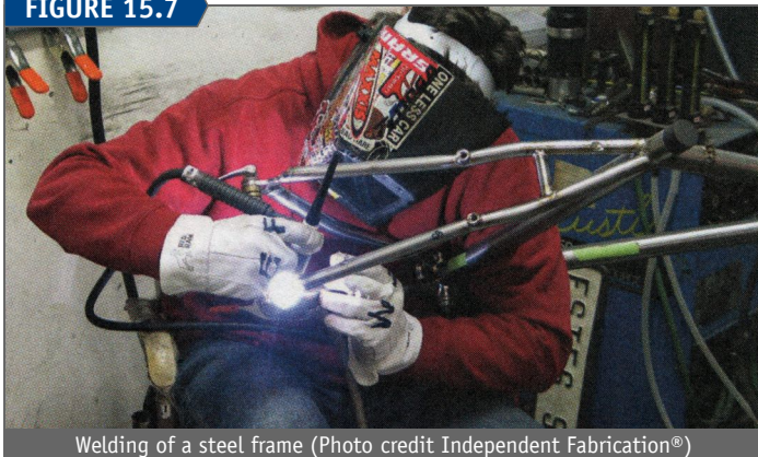
Welding of a steel frame (Photo credit Independent Fabrication®)
