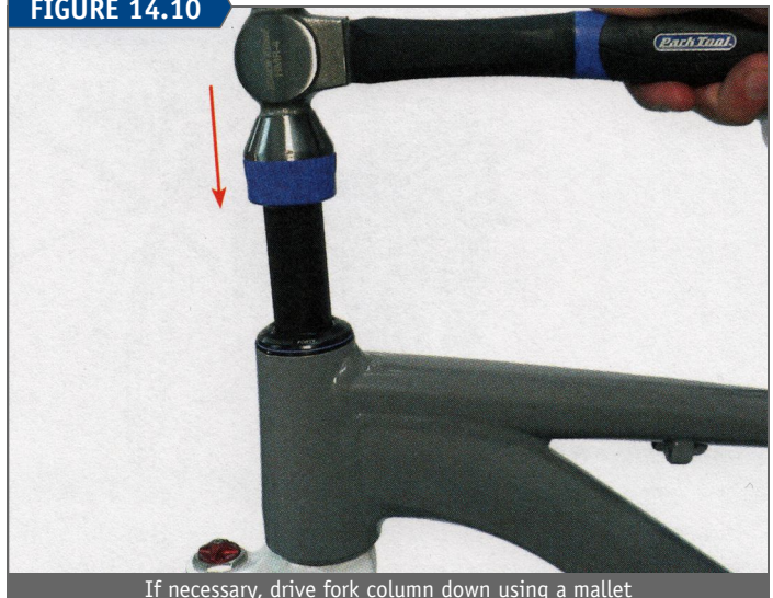
If necessary, drive fork column down using a mallet
