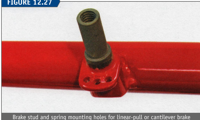
Brake stud and spring mounting holes for linear-pull or cantilever brake
