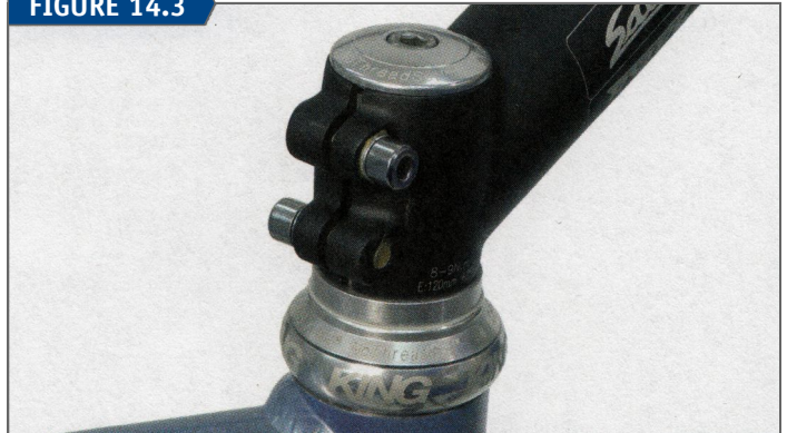
Threadless headset with external pressed cups, threadless stem, and top cap
