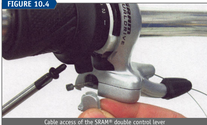
Cable access of the SRAM® double control lever
