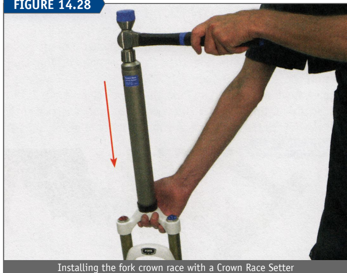
Installing the fork crown race with a Crown Race Setter
