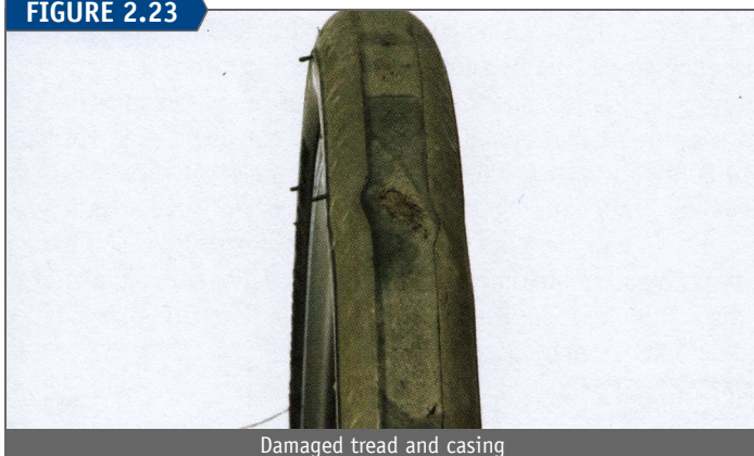
Damaged tread and casing
