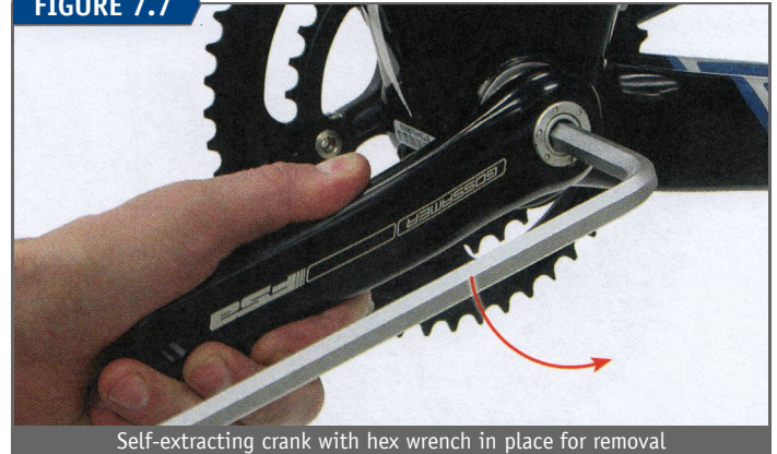
Self-extracting crank with hex wrench in place for removal
