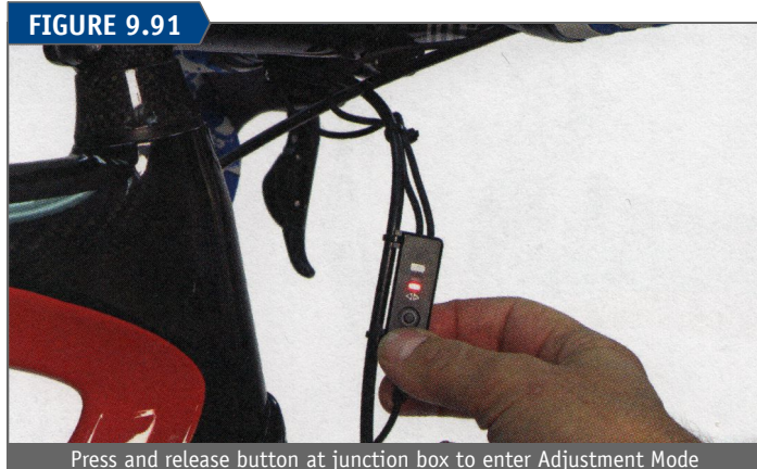
Press and release button at junction box to enter Adjustment Mode
