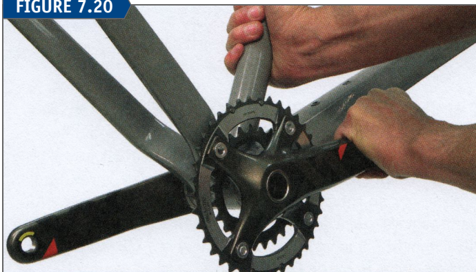
Hold frame with one hand and pull crank side-to-side checking for play
