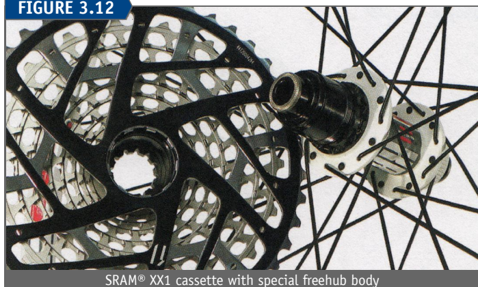
SRAM® XX1 cassette with special freehub body
