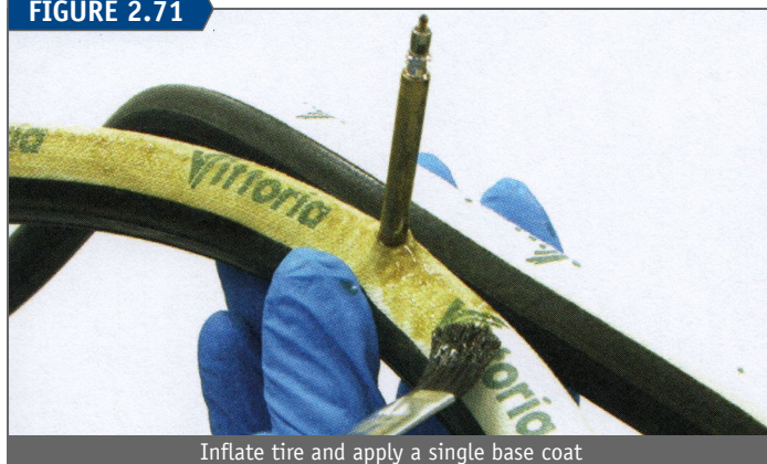
Inflate tire and apply a single base coat
