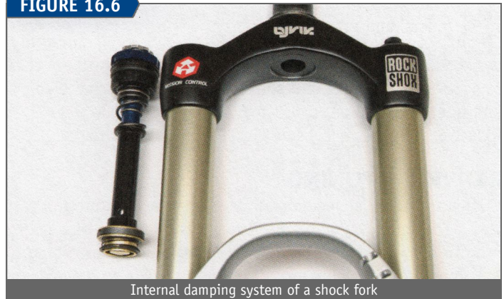
Internal damping system of a shock fork
