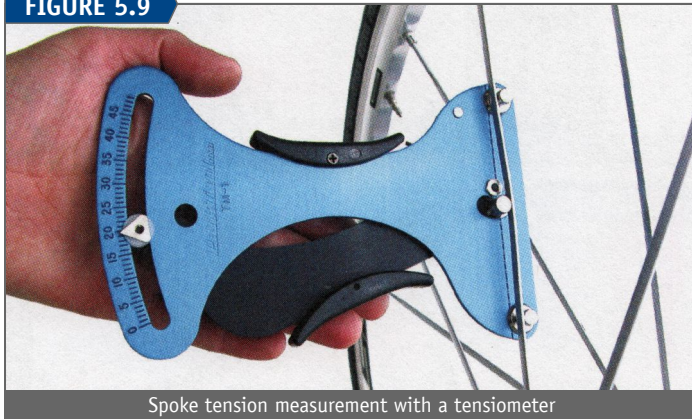
Spoke tension measurement with a tensiometer
