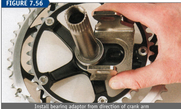
Install bearing adaptor from direction of crank arm
