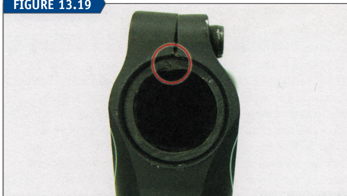
Cracked steering column from stem binder bolts
