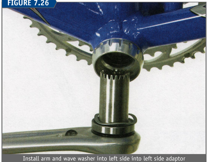
Install arm and wave washer into left side into left side adaptor
