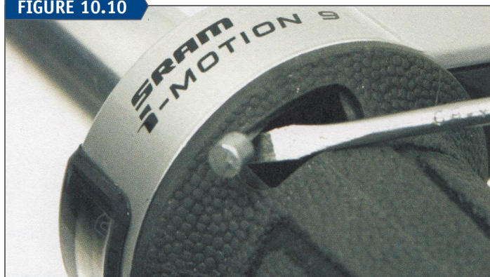
Remove cable from shifter
