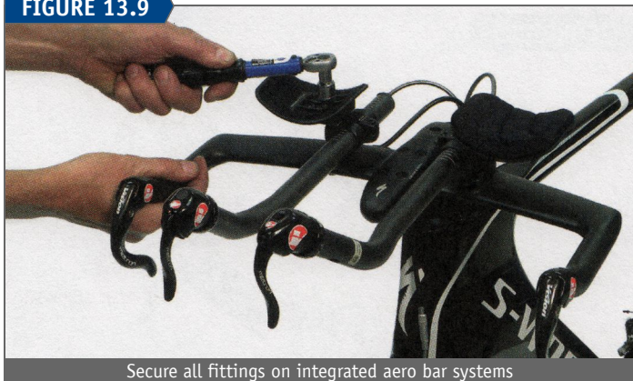
Secure all fittings on integrated aero bar systems
