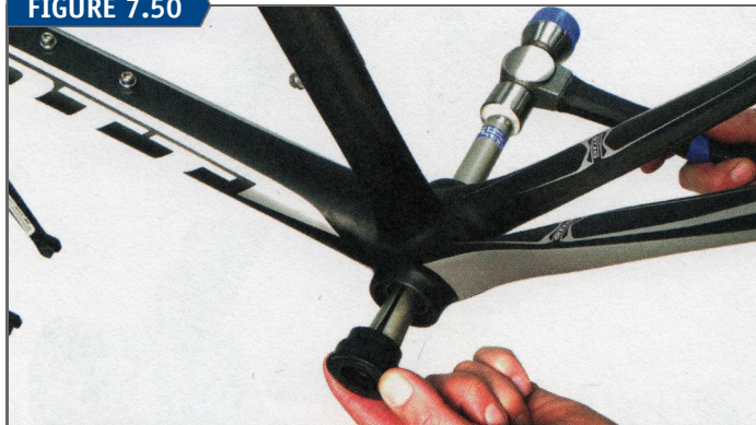
Remove bearing adaptor one at a time
