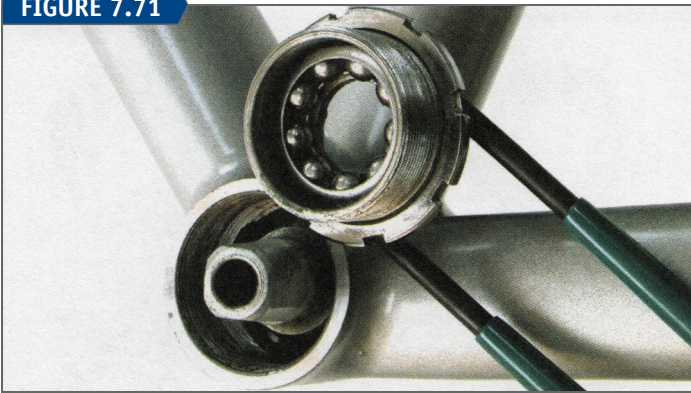
Remove adjustable cup (left side) locking, bearing cup and bearings
