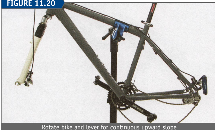
Rotate bike and lever for continuous upward slope
