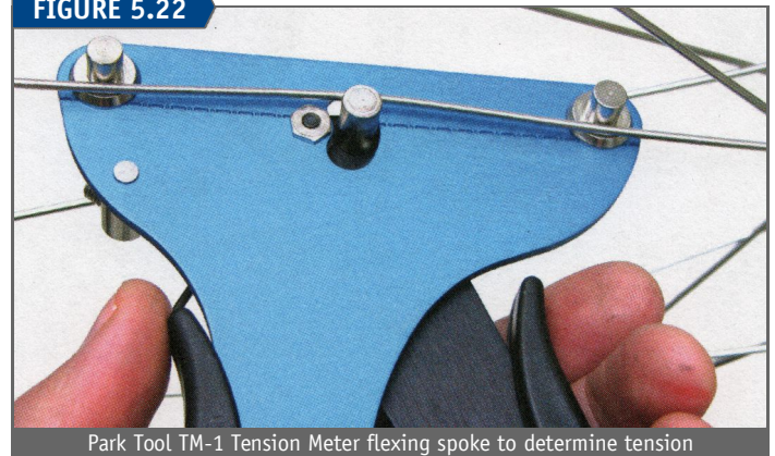
Park Tool TM-1 Tension Meter flexing spoke to determine tension
