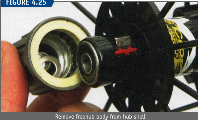
Remove freehub body from hub shell
