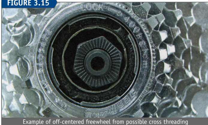
Example of off-centered freewheel from possible cross threading
