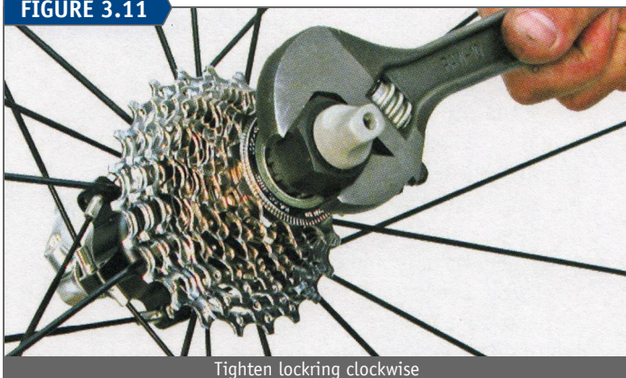
Tighten lockring clockwise
