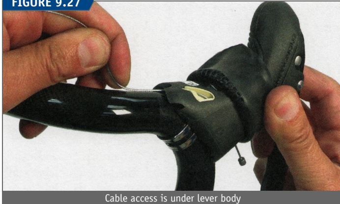
Cable access is under lever body
