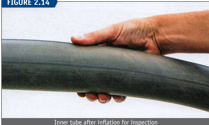
Inner tube after inflation for inspection
