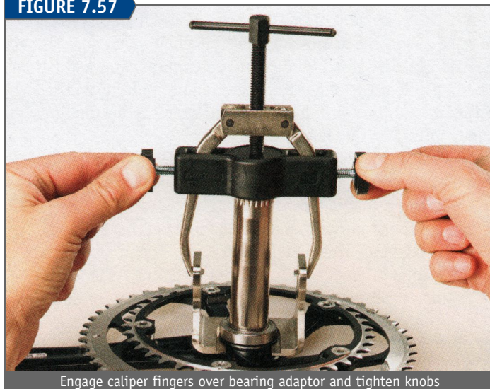
Engage caliper fingers over bearing adaptor and tighten knobs
