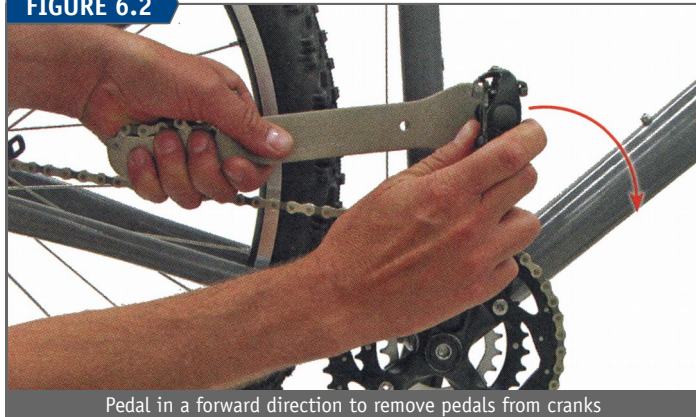
Pedal in a forward direction to remove pedals from cranks
