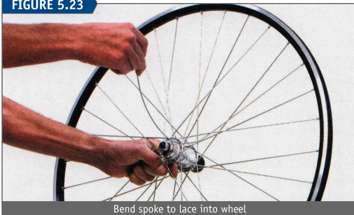
Bend spoke to lace into wheel
