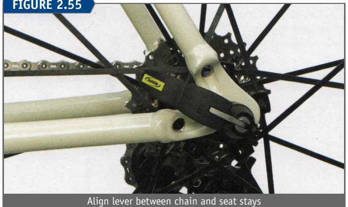
Align lever between chain and seat stays
