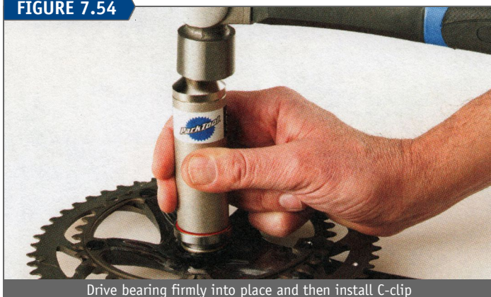
Drive bearing firmly into place and then install C-clip
