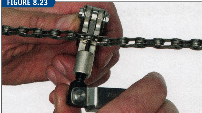
CT-6.3 used to set the Campagnolo 11-speed coupling pin
