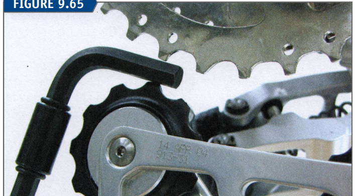
SRAM® and Shimano® Shadow setting for the upper pulley to largest cog
