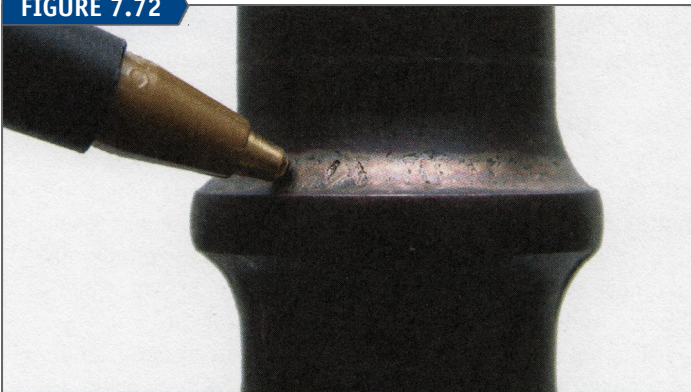
Trace bearing surfaces to feel for roughness and pits
