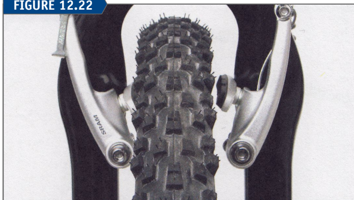
Misaligned wheel off to mechanic’s left
