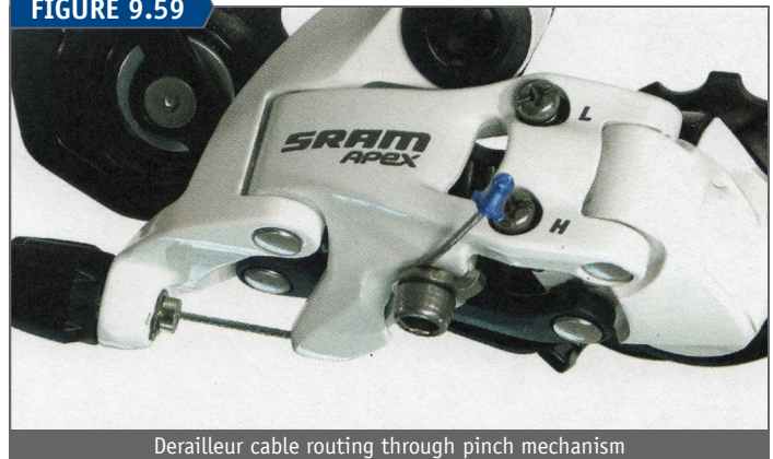
Derailleur cable routing through pinch mechanism
