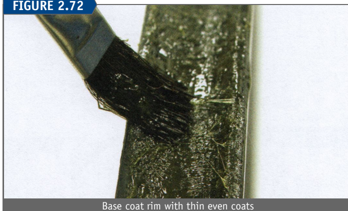
Base coat rim with thin even coats
