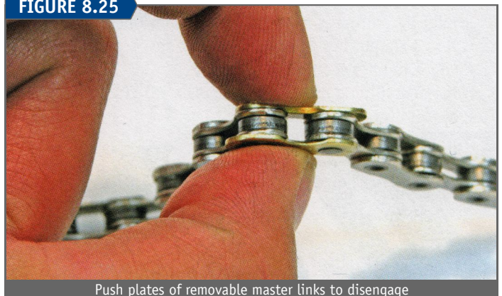
Push plates of removable master links to disengage
