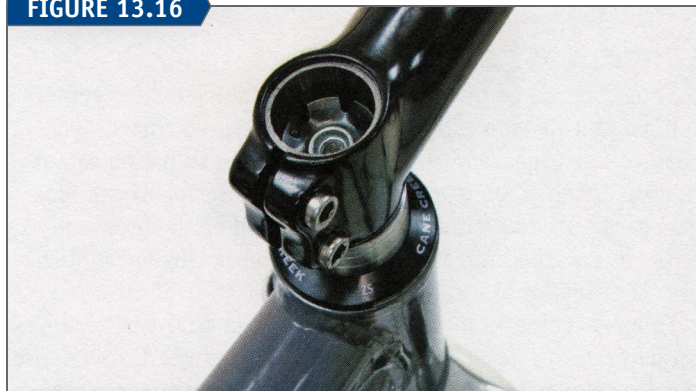
Threadless steering column recessed below threadless stem
