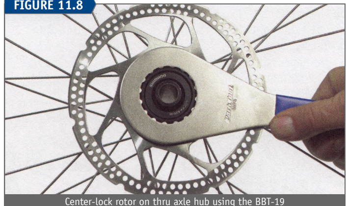
Center-lock rotor on thru axle hub using the BBT-19
