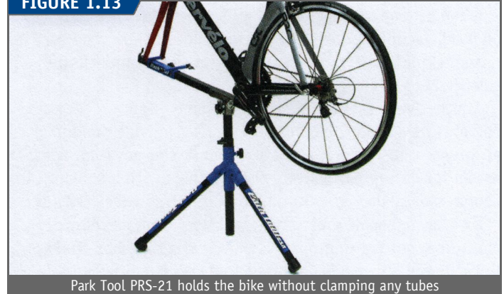
Park Tool PRS-21 holds the bike without clamping any tubes
