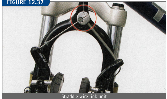
Straddle wire link unit
