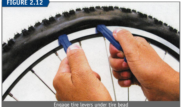
Engage tire levers under tire bead
