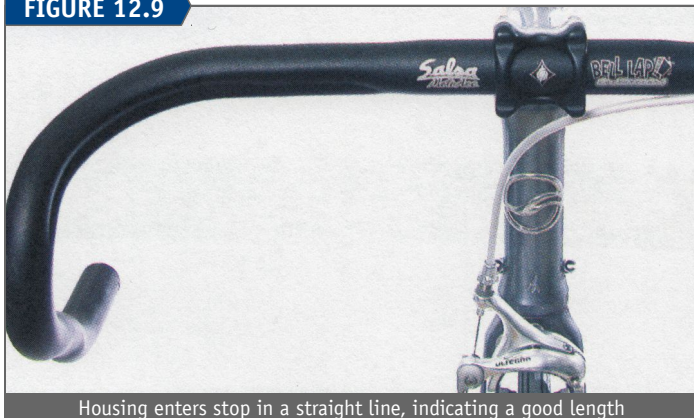
Housing enters stop in a straight line, indicating a good length
