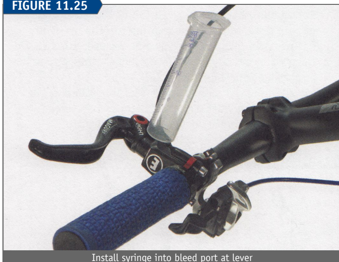
Install syringe into bleed port at lever
