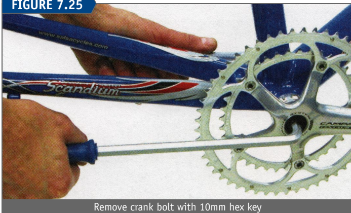
Remove crank bolt with 10mm hex key
