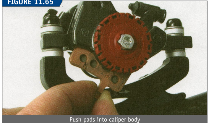
Push pads into caliper body
