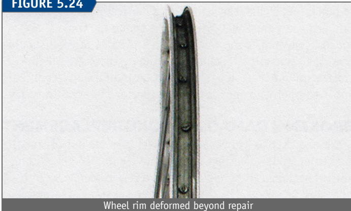
Wheel rim deformed beyond repair
