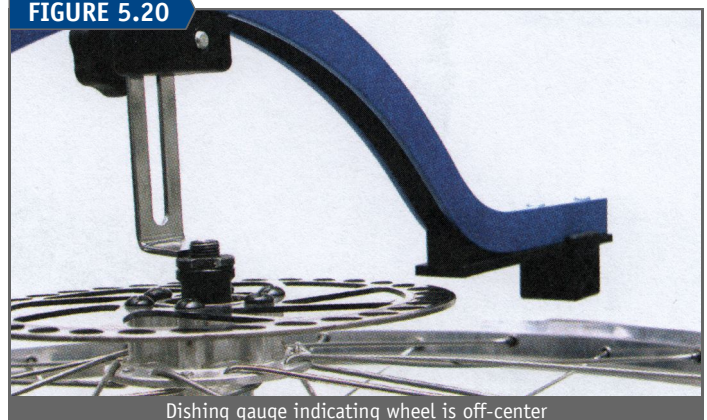
Dishing gauge indicating wheel is off-center
