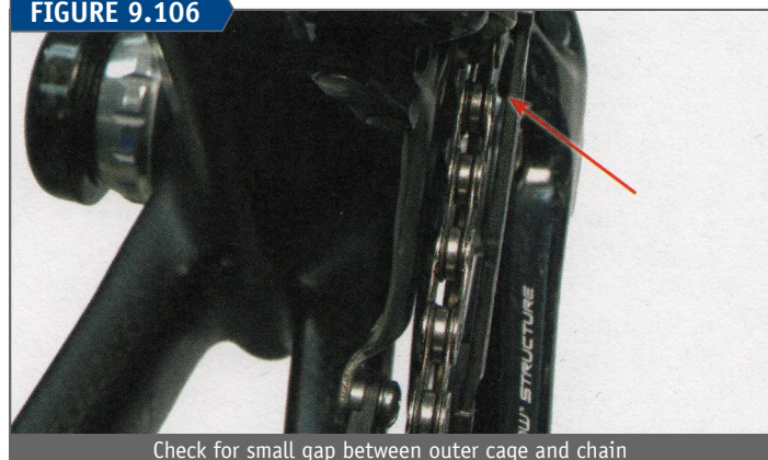
Check for small gap between outer cage and chain
