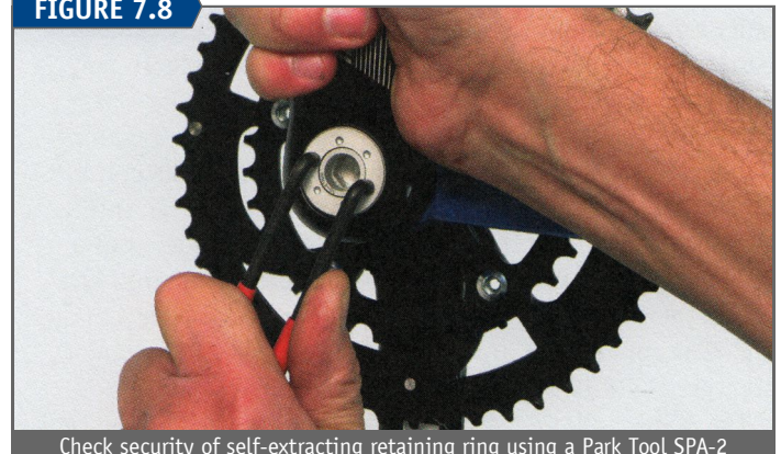
Check security of self-extracting retaining ring using a Park Tool SPA-2
