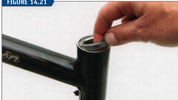
Removing the slip fit integrated bearing from an IS headset
