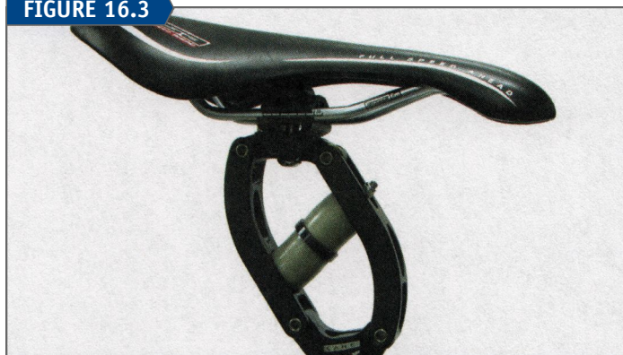
Elastomer spring system on a suspension seat post
