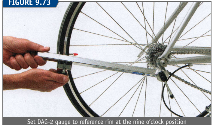
Set DAG-2 gauge to reference rim at the nine o'clock position
