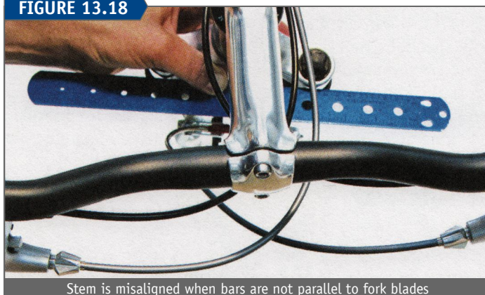
Stem is misaligned when bars are not parallel to fork blades
