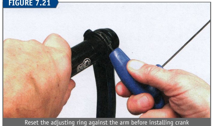
Reset the adjusting ring against the arm before installing crank
