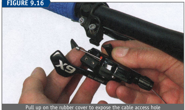
Pull up on the rubber cover to expose the cable access hole
