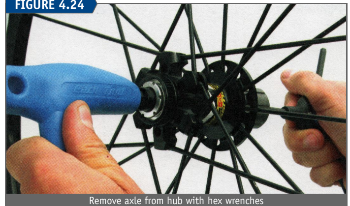
Remove axle from hub with hex wrenches
