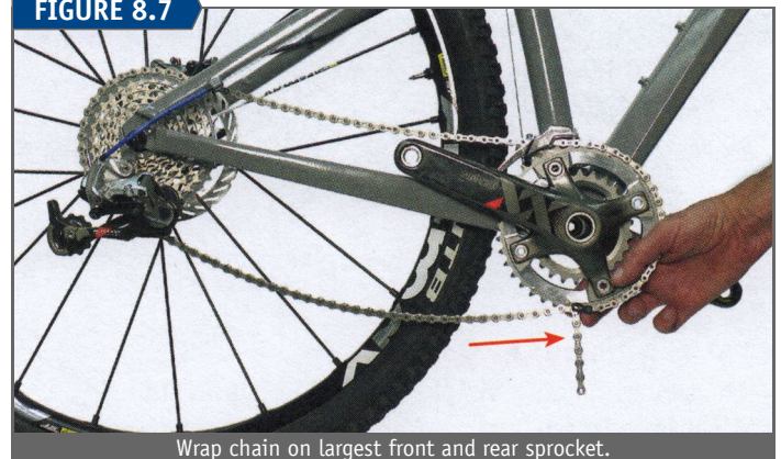
Wrap chain on largest front and rear sprocket.
