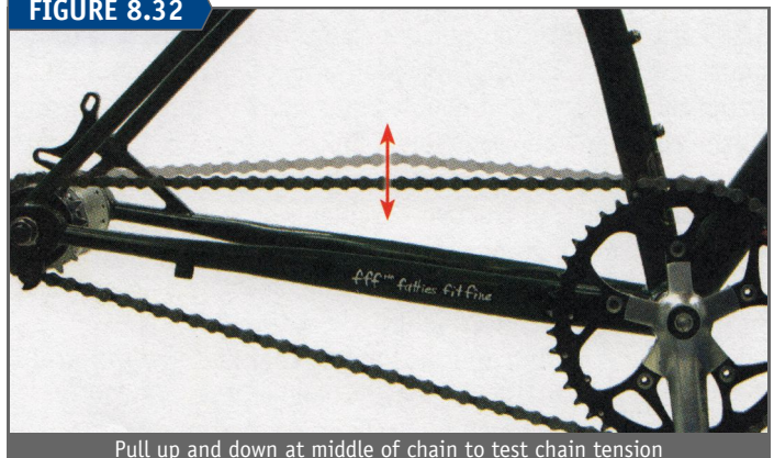
Pull up and down at middle of chain to test chain tension
