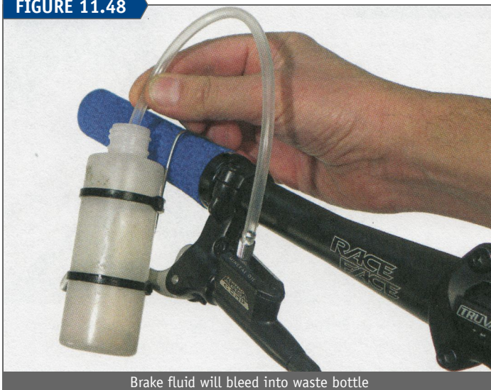
Brake fluid will bleed into waste bottle
