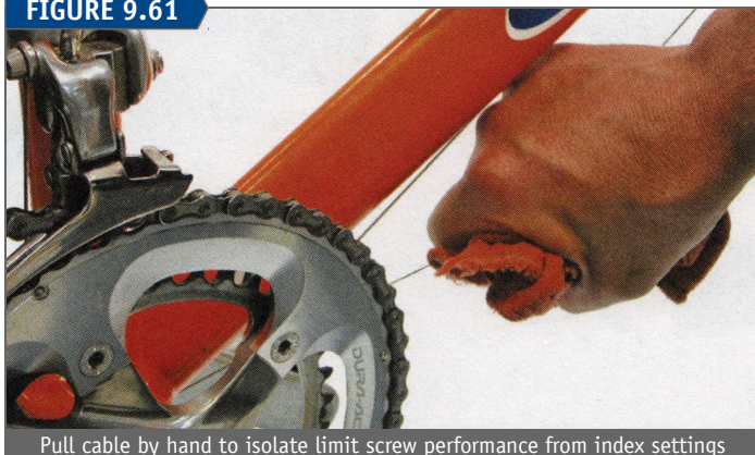
Pull cable by hand to isolate limit screw performance from index settings
