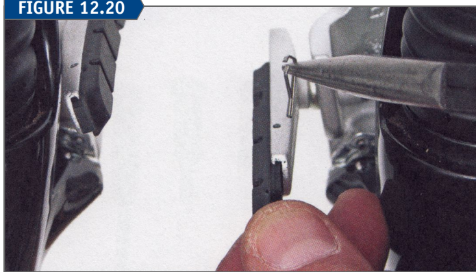
Pull cartridge pad toward back to remove pad from holder
