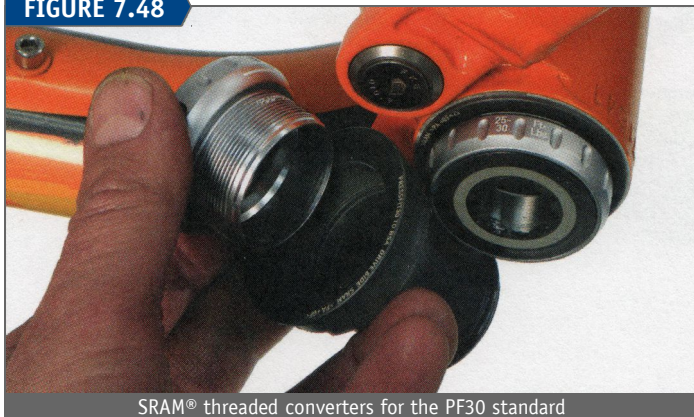
SRAM® threaded converters for the PF30 standard
