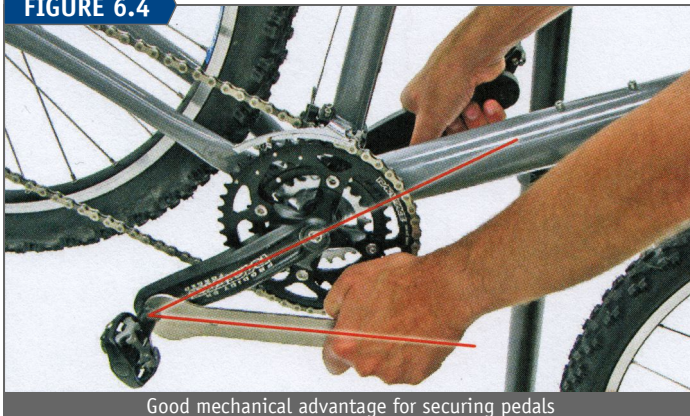
Good mechanical advantage for securing pedals
