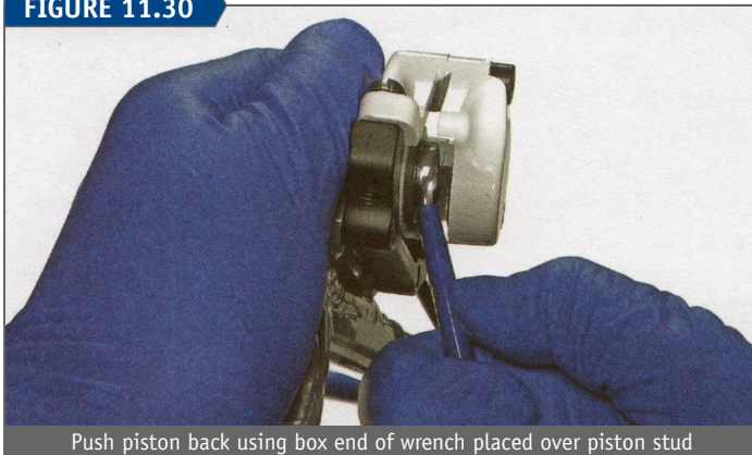
Push piston back using box end of wrench placed over piston stud
