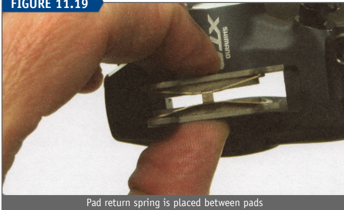
Pad return spring is placed between pads
