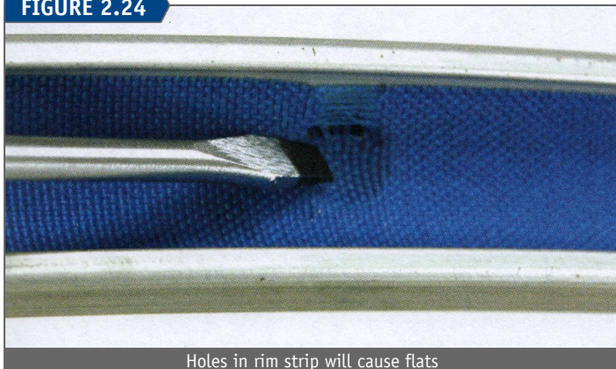
Holes in rim strip will cause flats
