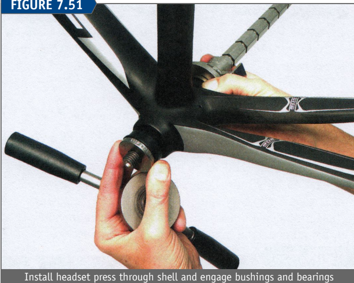
Install headset press through shell and engage bushings and bearings
