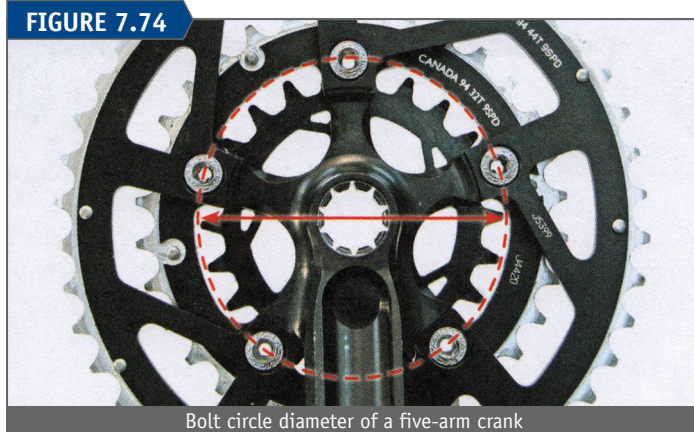
Bolt circle diameter of a five-arm crank
