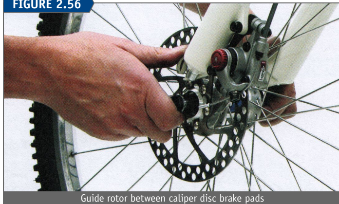
Guide rotor between caliper disc brake pads
