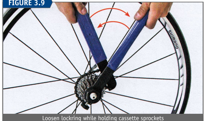
Loosen locking while holding cassette sprockets
