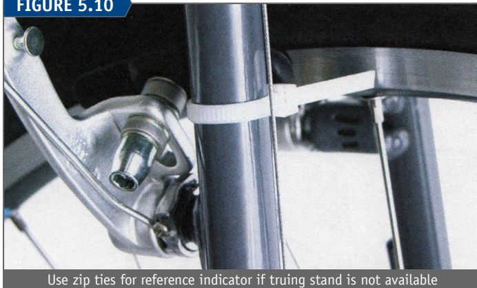
Use zip ties for reference indicator if truing stand is not available
