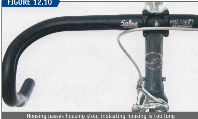
Housing passes housing stop, indicating housing is too long
