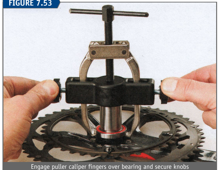
Engage puller caliper fingers over bearing and secure knobs
