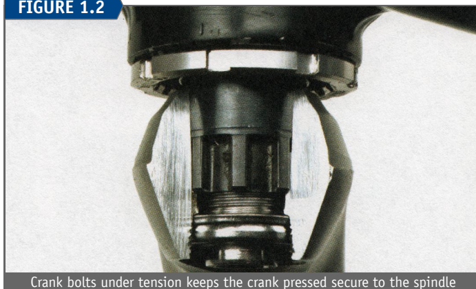
Crank bolts under tension keeps the crank pressed secure to the spindle
