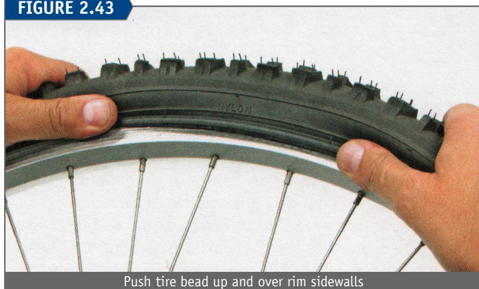
Push tire bead up and over rim sidewalls
