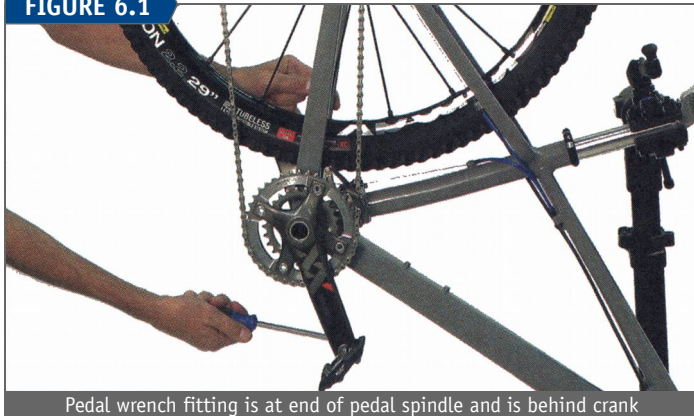
Pedal wrench fitting is at end of pedal spindle and is behind crank
