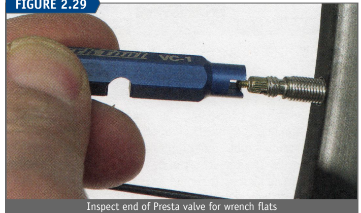
Inspect end of Presta valve for wrench flats
