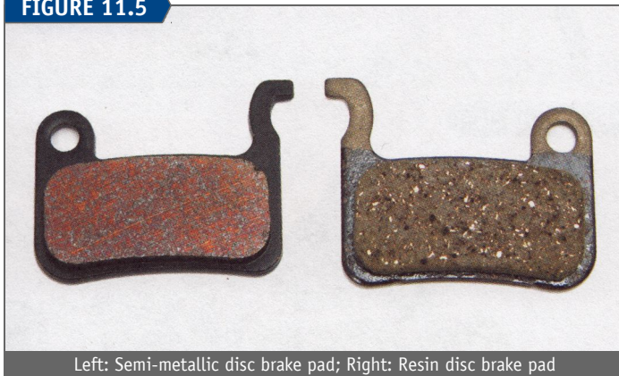
Left: Semi-metallic disc brake pad; Right: Resin disc brake pad
