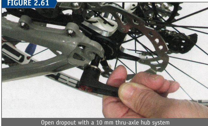
Open dropout with a 10 mm thru-axle hub system
