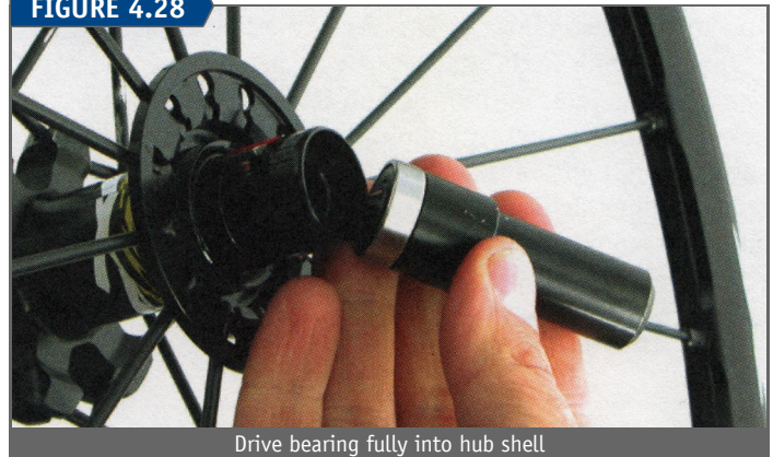
Drive bearing fully into hub shell
