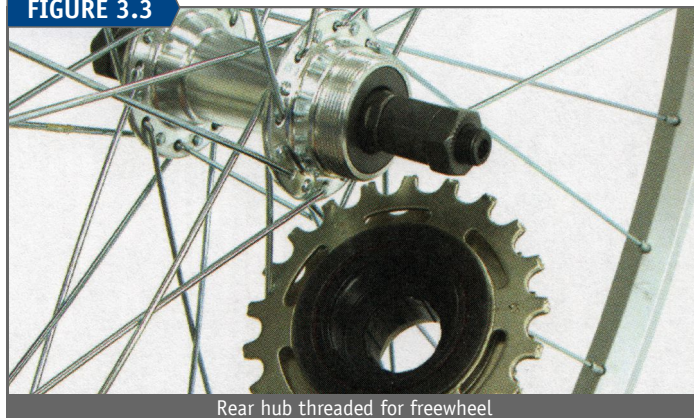
Rear hub threaded for freewheel
