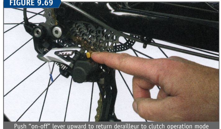
Push “on-off” lever upward to return derailleur to clutch operation mode
