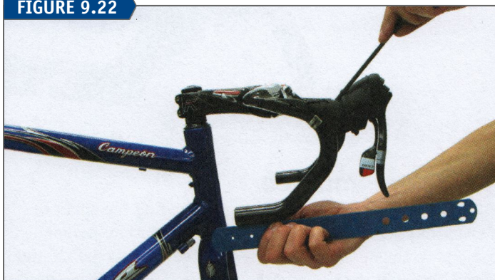
Align brake/shift levers relative to lower section of drop handlebars
