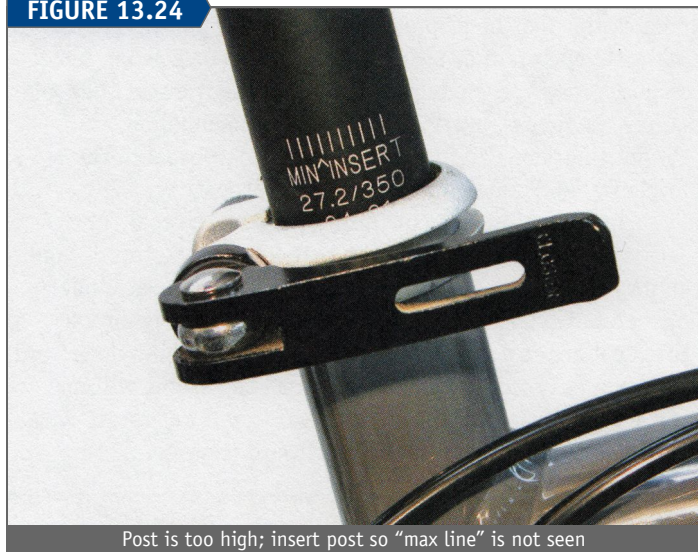
Post is too high; insert post so “max line” is not seen
