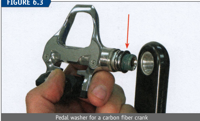
Pedal washer for a carbon fiber crank
