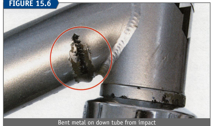
Bent metal on down tube from impact
