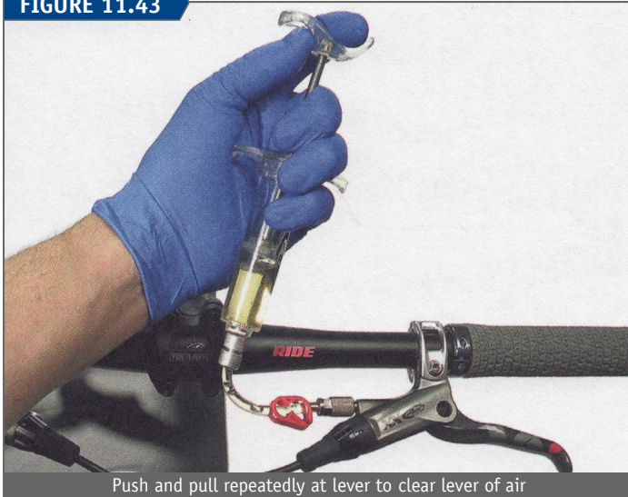
Push and pull repeatedly at lever to clear lever of air
