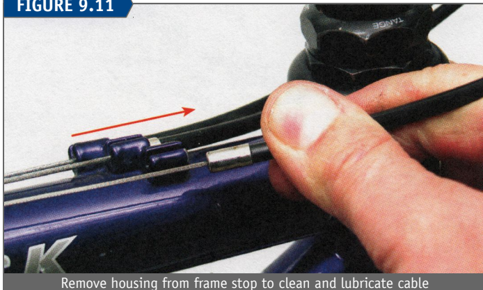
Remove housing from frame stop to clean and lubricate cable
