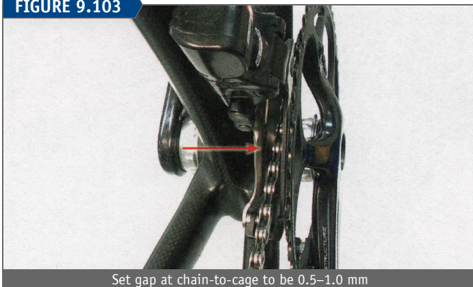
Set gap at chain-to-cage to be 0.5–1.0 mm
