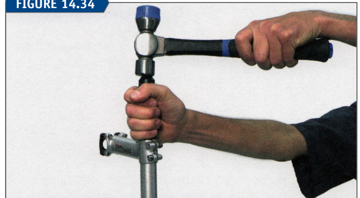
Using a stem to guide the TNS-1 and star nut straight with the column
