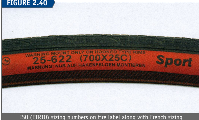
ISO (ETRTO) sizing numbers on tire label along with French sizing
