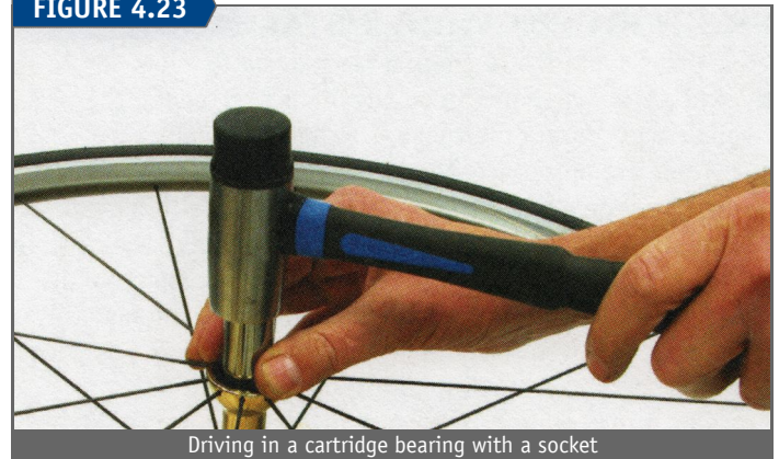
Driving in a cartridge bearing with a socket
