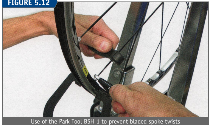
Use of the Park Tool BSH-1 to prevent bladed spoke twists
