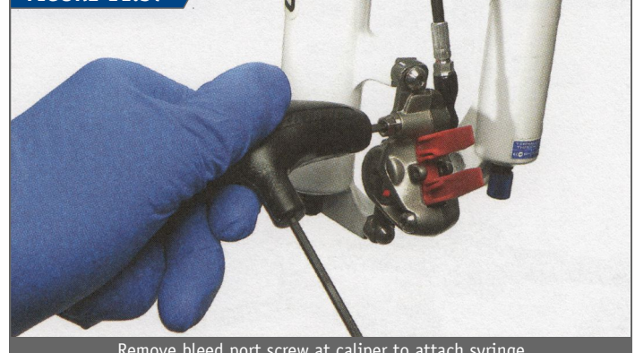
Remove bleed port screw at caliper to attach syringe
