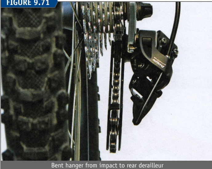
Bent hanger from impact to rear derailleur
