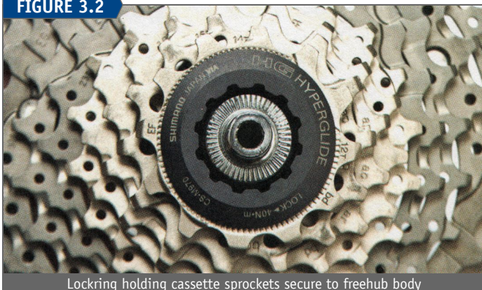
Lockring holding cassette sprockets secure to freehub body
