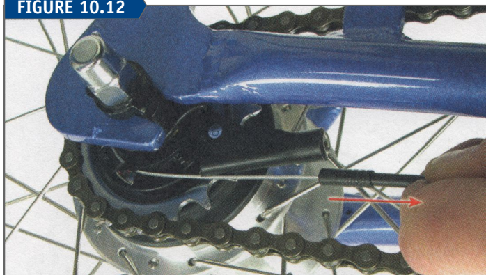
Release cable from housing stop to detach anchor from cassette joint
