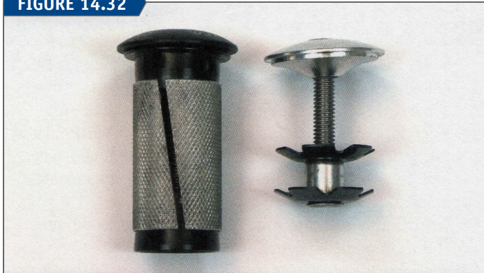
Compression plug on the left. Star nut with bolt and top cap on the right.
