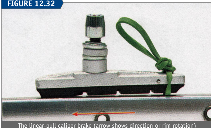
The linear-pull caliper brake (arrow shows direction of rim rotation)
