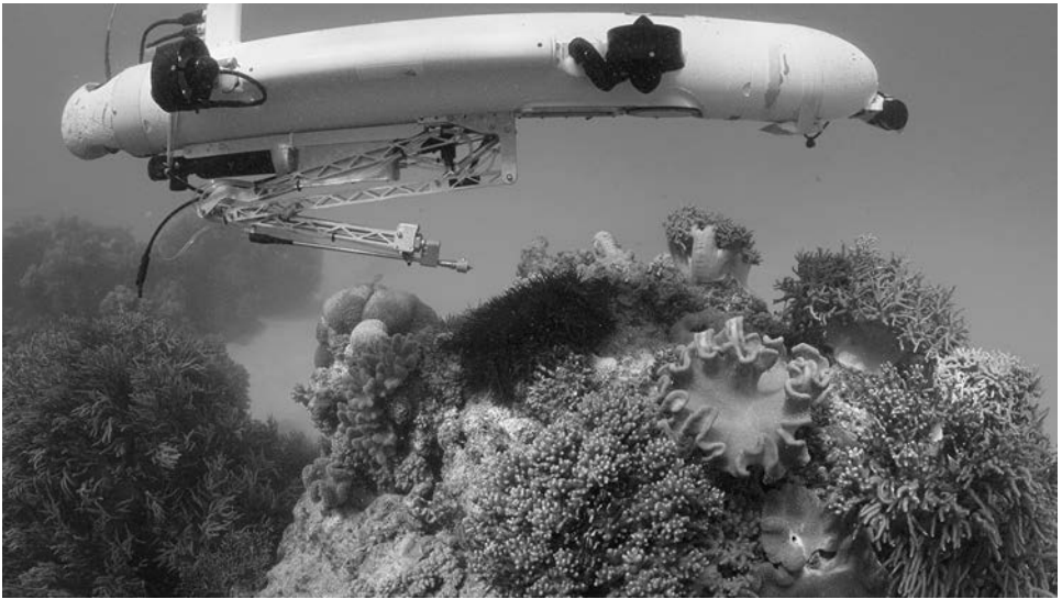
FIGURE 7.1. Researchers Matthew Dunbabin and Feras Dayoub (unseen) completing field trials of their COTS robot, which can navigate difficult reefs, detect COTS, and deliver a fatal dose of bile salts. Credit: Richard Fitzpatrick for QUT. Used with permission.
