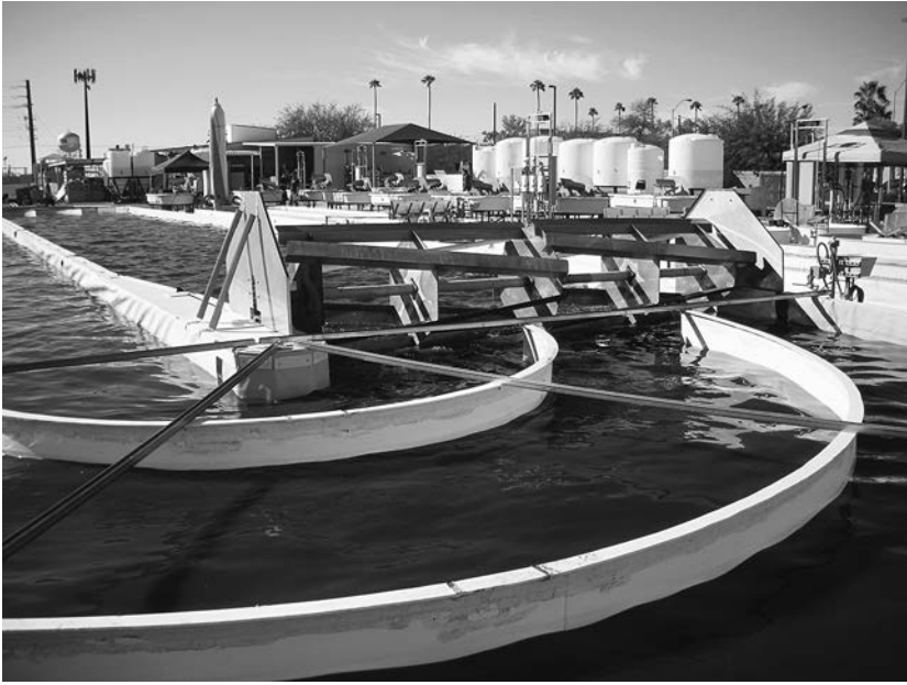
FIGURE 14.2. An Algae Raceway Integrated Design (ARID) Raceway (around thirty thousand liters) on AzCATI's precommercialization testbed facility. Photo by author.
