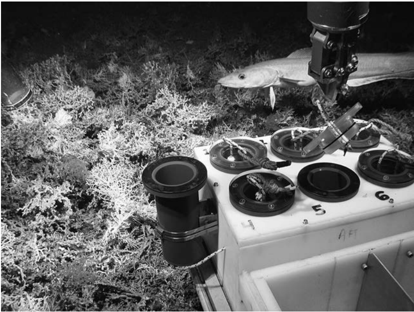
FIGURE 7.3. Subsea image showing the ROV manipulator opening a tube for a coral sample to be placed inside while a curious ling looks on. Courtesy of J Murray Roberts.
