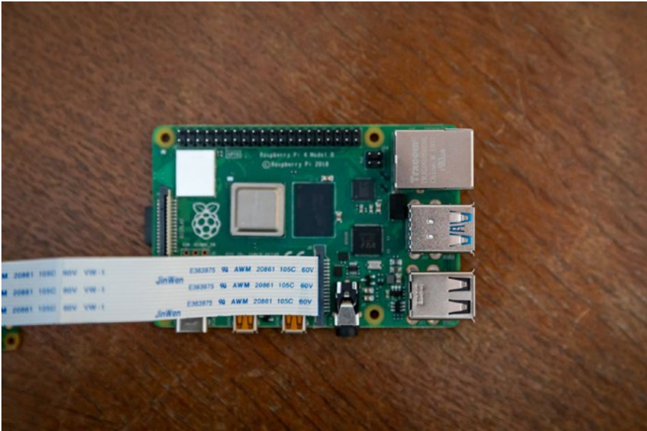
Figure 11-3. Pi Camera ribbon cable installed on the Pi
