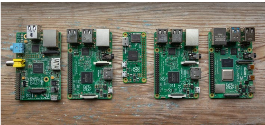
Figure 1-1. Raspberry Pis, from left to right: Pi 1, Pi 2, Pi Zero, Pi 3, Pi 4
