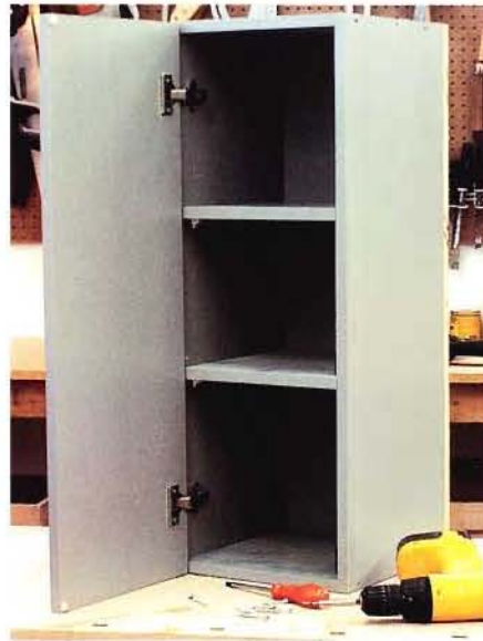
MPB sheets come in dozens of colors and simulated woodgrain finishes. Many manufacturers can also supply a matching edge tape.
