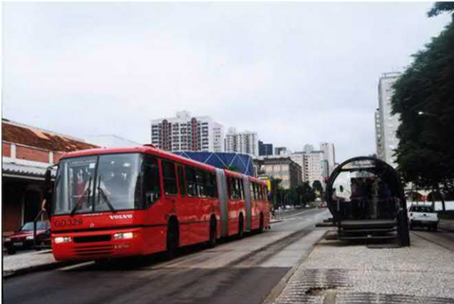
FIGURE 4.2 BRT vehicle and tubular bus platform.
