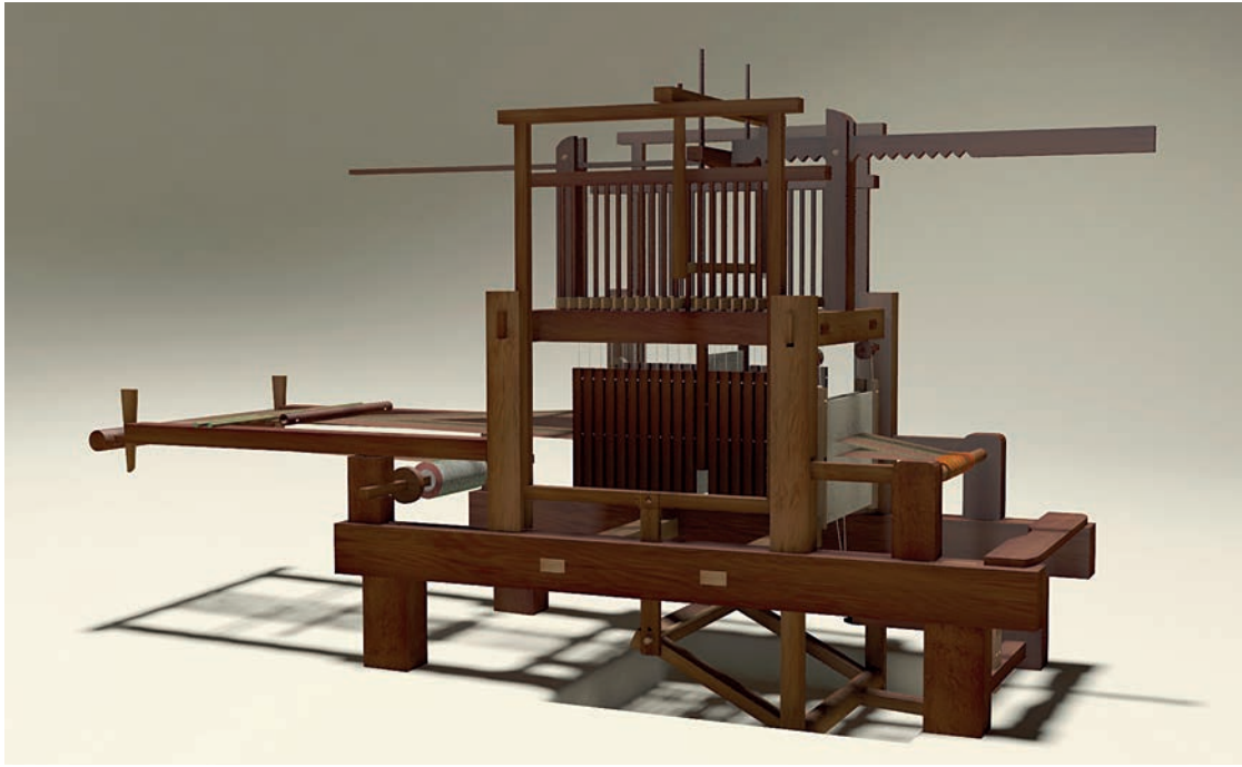
FIGURE A.6. Reconstruction of Laoguanshan loom. Courtesy of China National Silk Museum, Hangzhou.
