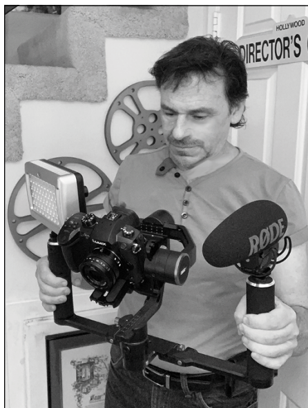
FIGURE 14-8: The author/director using the Fig Rig on-set (left); the FeiyuTech stabilizer with PRL camera light and the Røde directional mic attached to the gimbal handles (right).
