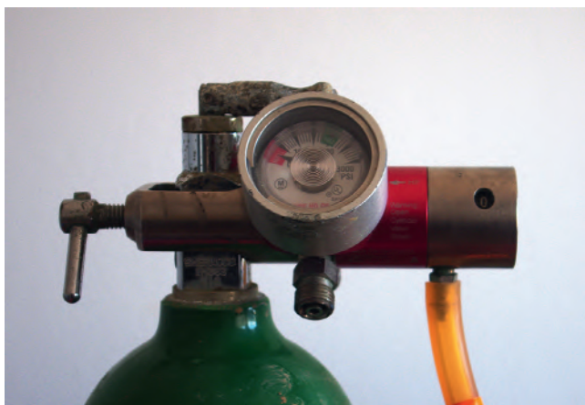
• Figure 28.3 Oxygen pressure regulator with a pressure gauge and an integrated flowmeter that may be used to supply a portable anesthesia machine through the attached hose or may be connected to an oxygen demand valve.
