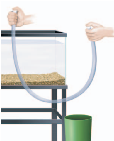
Fill the siphon with water and use your thumbs to block both ends.
