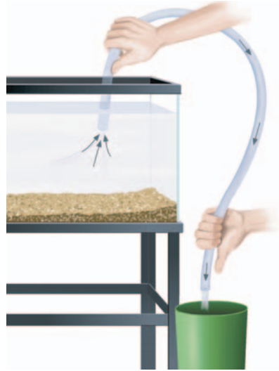
Place one end in the tank and one end in the bucket, and water will flow.
