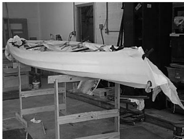
Skin clamped in place
