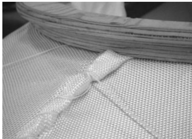
Deck seam at coaming
