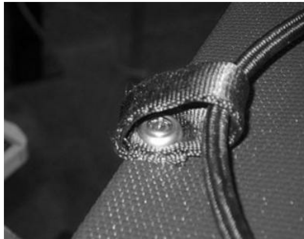
Finished tie down point
