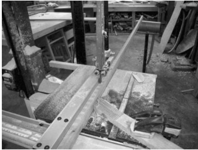
Sawing the strips
