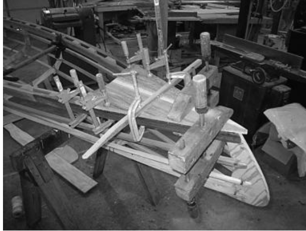
Breasthook clamped in place
