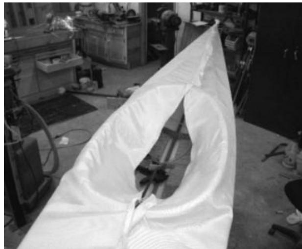
Coaming ring in place
