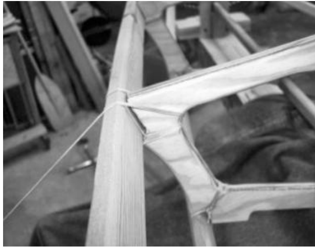
Lashing the frame
