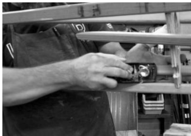
Using a block plane to clean up the stringers
