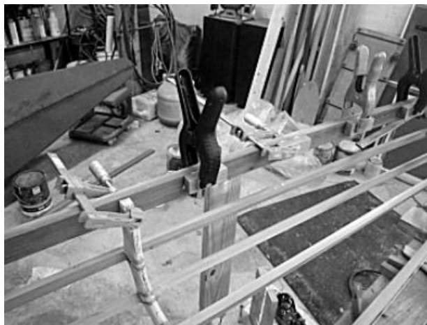
Gluing spacer blocks in place
