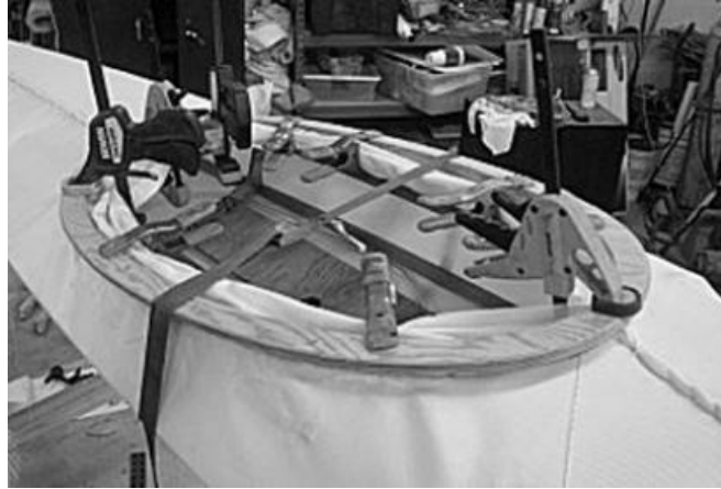
Coaming clamped in place
