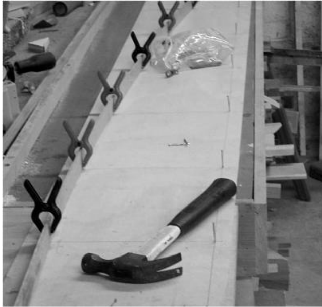
An example of using a batten being used to draw a curve
