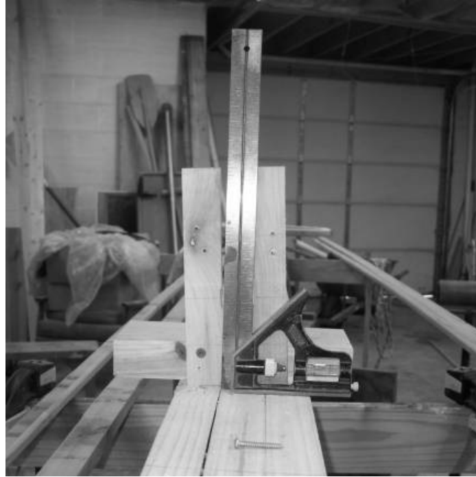
Checking alignment of the bracket
