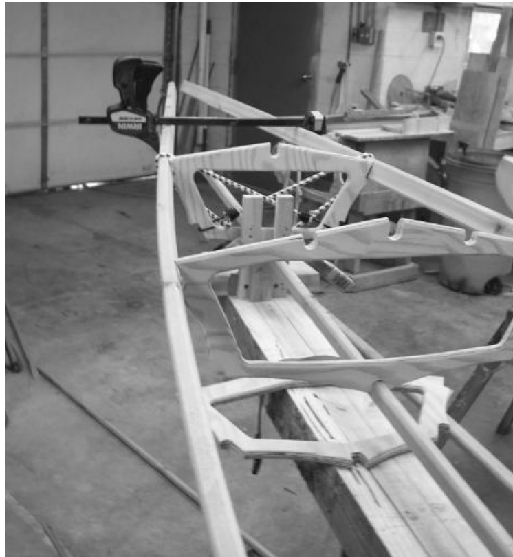
Gunwale ends clamped
