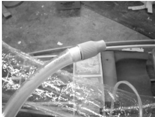
NRS valve glued on vinyl fill tube
