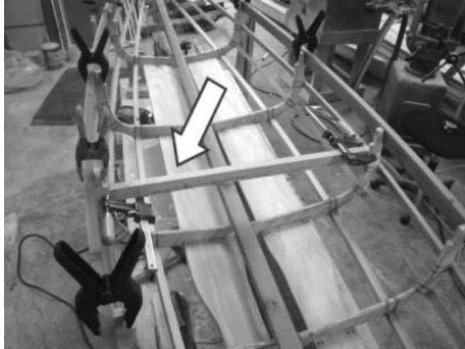
Temporary thwarts or bracing
