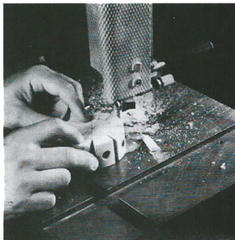
Fig. 1. Cut out the wedges in the engine block to create the cylinders. Make the cuts with a bandsaw or scroll saw.
