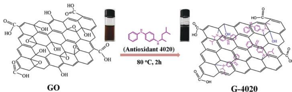
Figure 5.44. Schematic of reduction and functionalization of graphene oxide by antioxidant. [Adapted, by permission, from Zhong, B; Dong, H; Luo, Y; Zhang, D; Liu, F, Composites Sci. Technol. , 151 , 156-63, 2017.]
