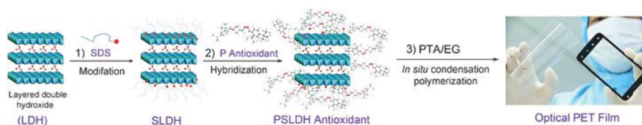
Figure 5.25. Schematic representation of fabrication of the hybridized antioxidant and its in situ addition into PET. [Adapted, by permission, from Sun, S; Wang, L; Song, P; Ding, L; Bai, Y, Chem. Eng. J. , 328 , 406-16, 2017.]
