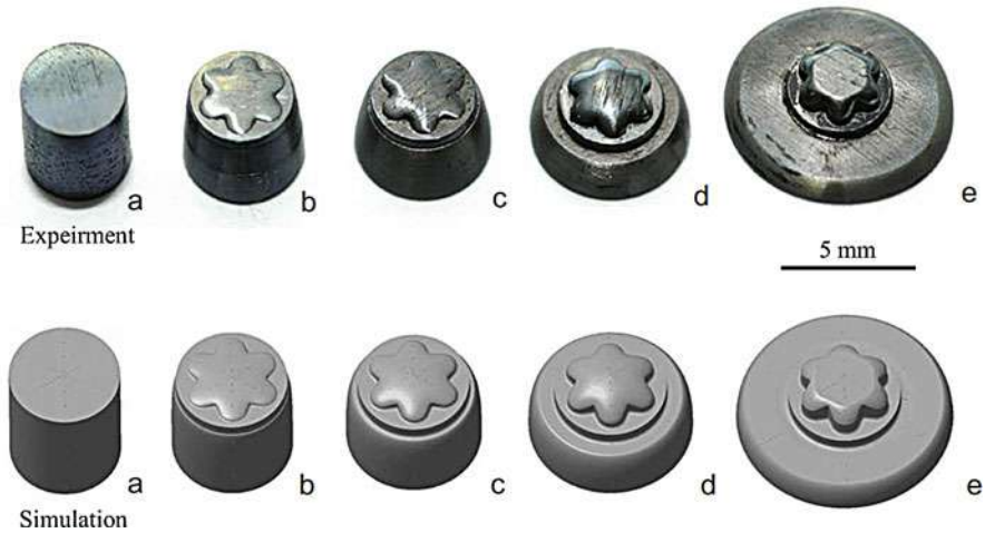
Fig. 8 Top row: the shapes of a miniature gear component achieved by the superplastic forming of the \text{La}_{61.4}\text{Al}_{15.9}\text{Ni}_{11.35}\text{Cu}_{11.35} metallic glass in experiments. Bottom row: the shapes obtained from the simulation with the use of a metallic-glass constitutive model at high homologous temperatures (Thamburaja and Ekambaram 2007). (a) Initial shape, (b–d) intermediate shapes, and (e) final shape. The forming process is conducted at an ambient temperature of 432 K with the use of a pre-made die (Ekambaram et al. 2010)
