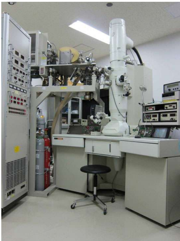
Fig. 1 Example of a transmission electron microscope (TEM) combined with a low-energy ion accelerator at Shimane University in Japan (Arakawa et al. 1999). Using this instrument, the dynamic behavior of local structures such as defects within solids can be monitored with nanoscale spatial resolution and recorded with 30 frames per second, in response to ion irradiation under heating, cooling, or deformation
