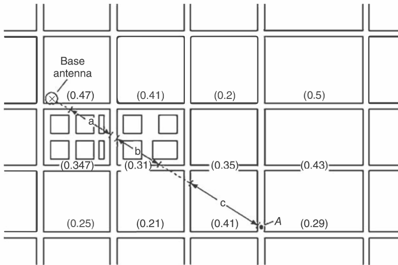
FIGURE 4.2.1.4.1 A simple method of estimating building blocks.
