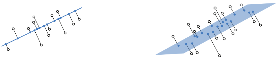
Figure 1.14 Two toy datasets consisting of two-dimensional (left panel) and three-dimensional (right panel) input data, shown as hollow black circles. The data in each case is projected onto a lower-dimensional subspace, and is effectively lowered a dimension while retaining a good amount of the original data's structure.
