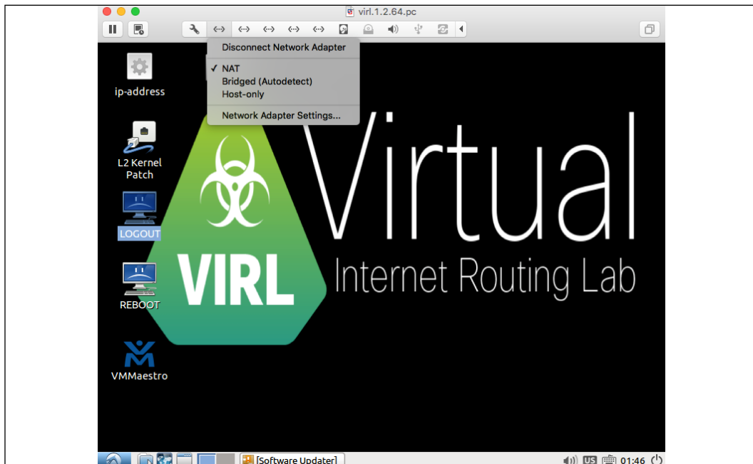
Figure 2: VIRL Ethernet adapter 1 changed to NAT
