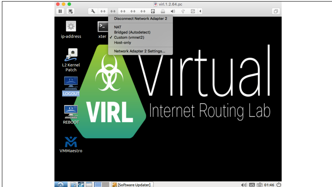
Figure 3: VIRT Ethernet adapter 2 connects to VMNet2
