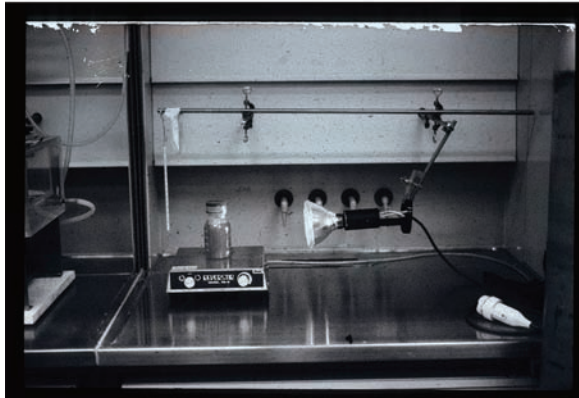
PLATE 3 "Stuff that does something." Slides used in presentations by Dieter Oesterhelt, presumably mid-1970s. Top, photo of cuvette filled with purple membrane material suspended with salt solution and ether. Bleaching from purple to yellow was achieved by illumination with a focused light beam, demonstrating the material's reactivity (photoeffect). Similar images demonstrating material activity were frequently shown in presentations by bacteriorhodopsin researchers. Bottom: Experimental set-up to demonstrate photoeffects, e.g., in lectures. Images reproduced with permission of D. Oesterhelt, Martinsried.
