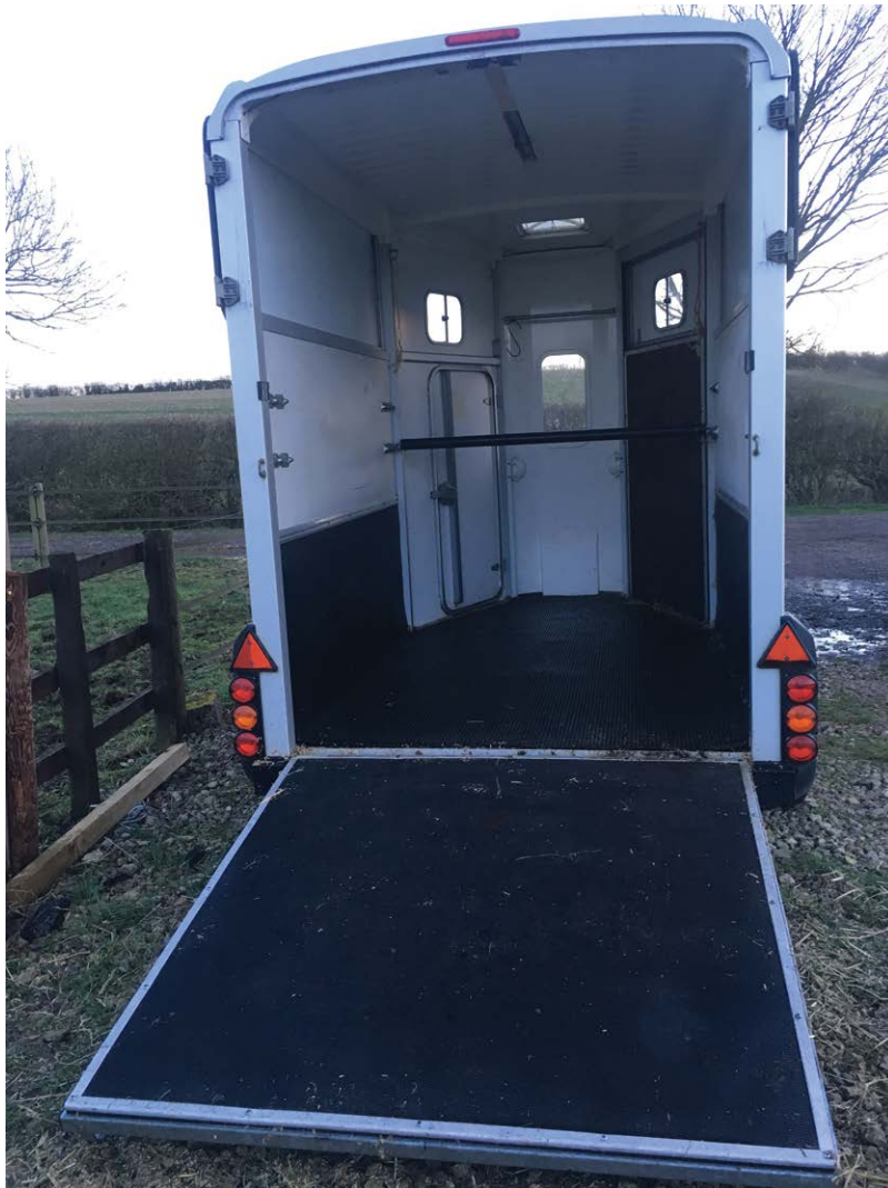
Fig. 17.1. A typical horse box with common features that horses may find aversive. First, the horse has to step up onto the ramp, which may be an action naturally avoided. Second, the ramp is at an angle and so the lower joints of the limb may need to hyperextend, which may be uncomfortable. The black surface will also naturally be avoided as may be a surface associated with vibrations underfoot. It must also be recognized that the horse box is a very novel looking and potentially smelling, enclosed environment associated with isolation in a dead-end space, all of which are features that horses will naturally avoid; this is further exacerbated by high contrast features making the transition from inside to outside very strong. Finally, the surface may also be slippery and not provide a solid grip. Failure to appreciate and address effectively how these features affect a horse can lead an owner to use punishment on the horse who hesitates or refuses to enter, which will add a further learned negative association to the box, resulting in horses who are traumatized at the prospect of loading or traveling.
