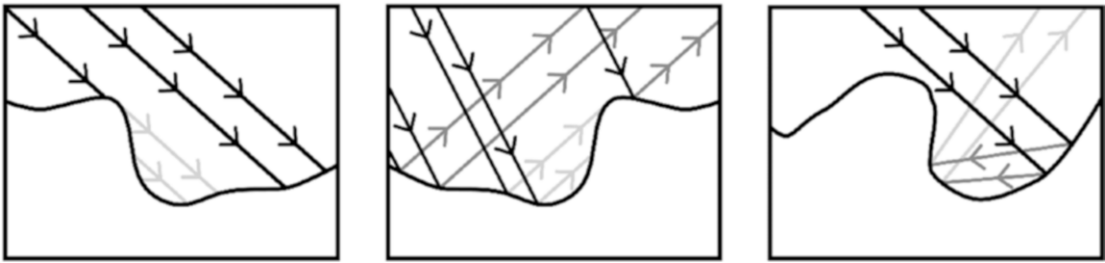
Figure 8-11. Respectively shadowing and masking approximations used by the theory, as opposed to reality (light bounces)
