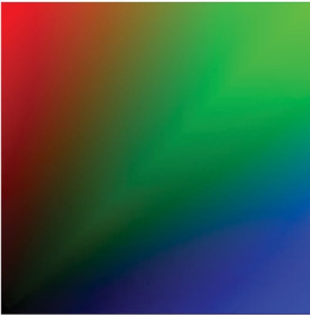
Figure 3-3. Interpolation of vertex colors by the rasterizer
