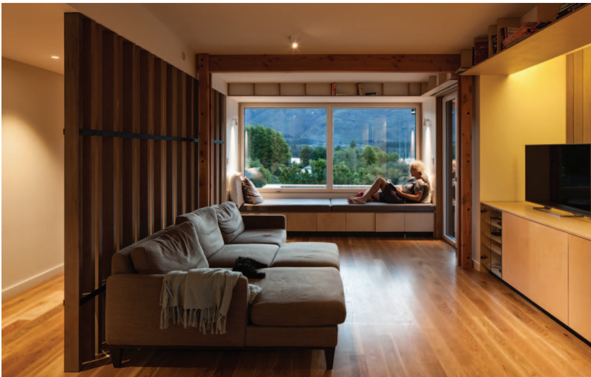
Lighting in a Passive House, Wanaka, has electric task lighting and daylight in the bay window, indirect light washing the walls behind the television creating volume and diffuse light, with general down lighting in the hallway (Photo: Simon Devitt).
