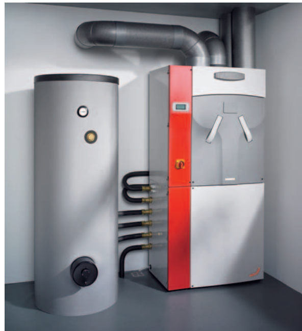
Example of a combined domestic hot water and heat recovery ventilation compact unit (see figure on p. 103 for schematic) that recovers waste heat from the exhaust air to heat hot water via a small heat pump (Photo: Zehnder Group).
