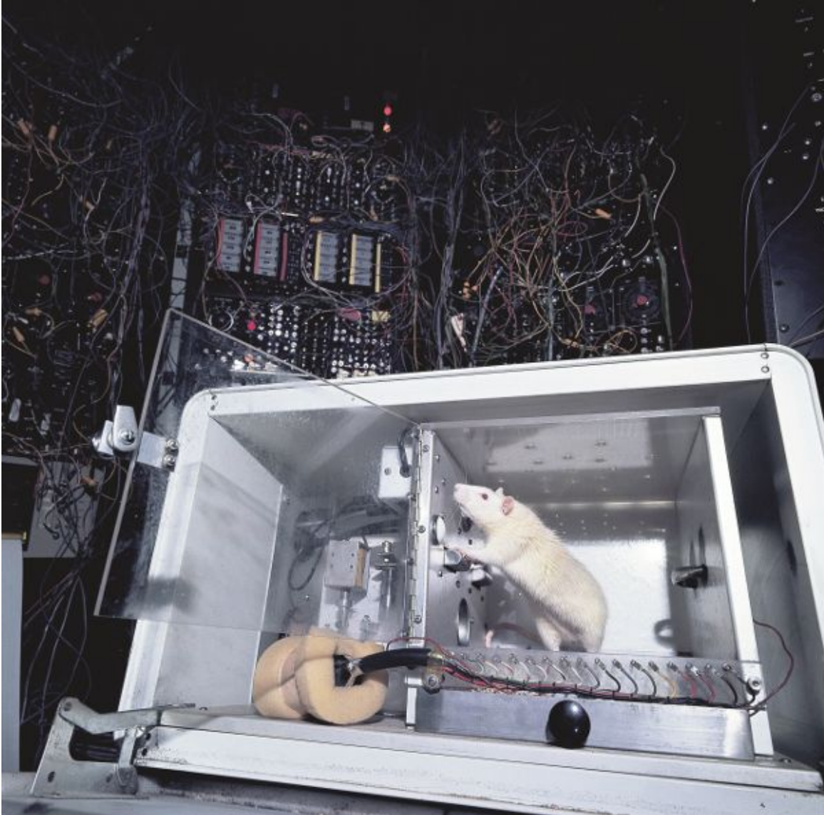
Figure 5.14. Rats in a Skinner box. To test various theories of animal learning, rats are often placed in “Skinner boxes,” where they have to take an action (here, pressing a button) to get a reward of food or water. (Photo credit: Walter Dawn/Getty Images)
