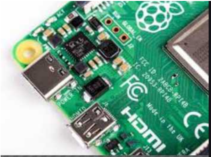
Raspberry Pi 4 showing HDMI port
