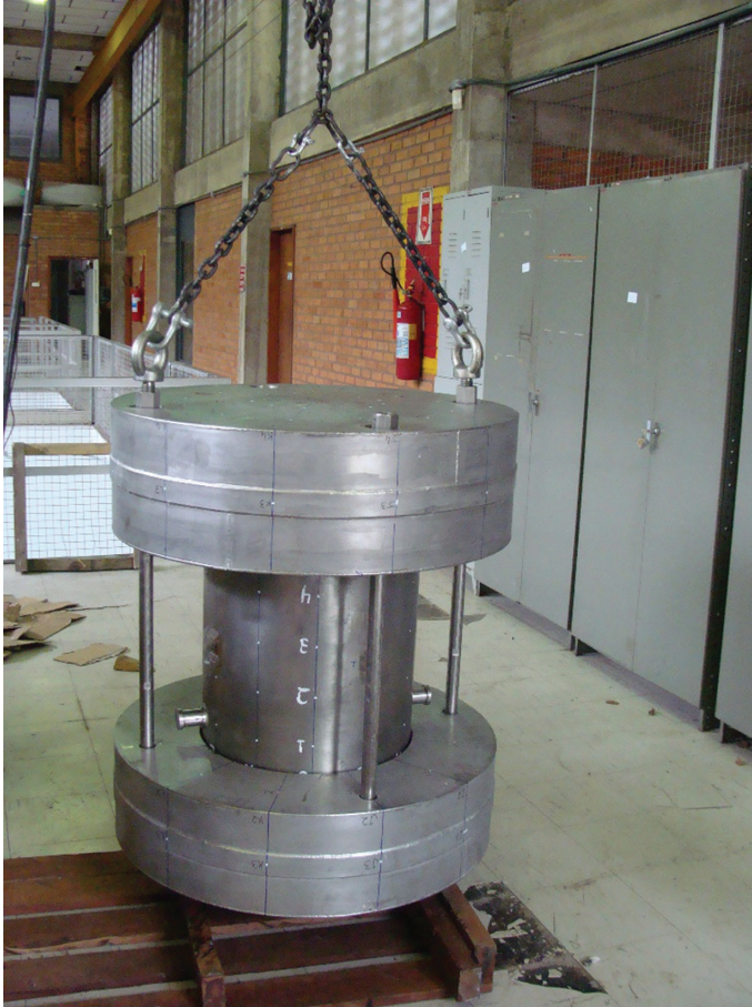
FIGURE 6.2 Photography of spent fuel transport and storage RLA4018 design by CDTN.
