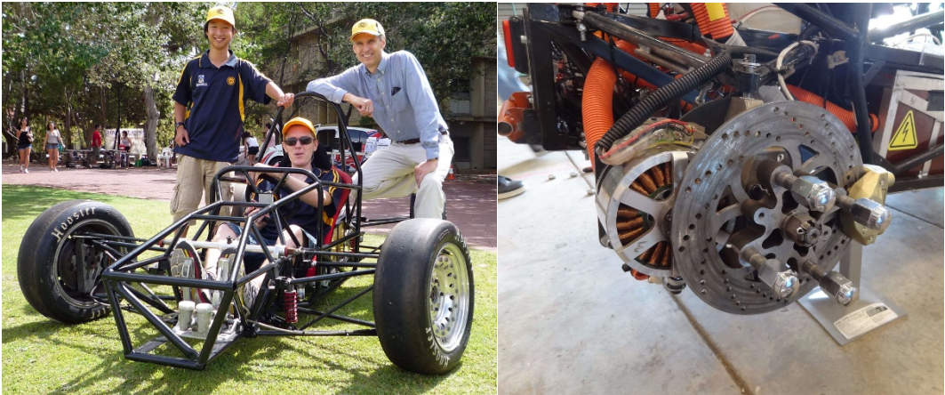
Figure 14.2: J. Wan, I. Hooper and T. Bräunl with the 1st generation Formula SAE Electric car (left) and wheel hub motors of 2nd generation car (right)
