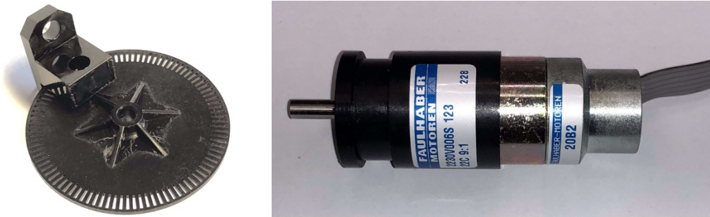
Figure 1.3: Incremental encoder (left); motor with encapsulated gearbox and encoder (right)
