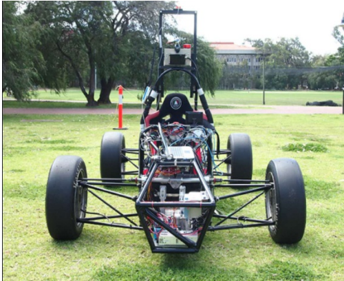
Figure 14.7: Fully autonomous Formula SAE Electric vehicle with sensors above the driver's seat
