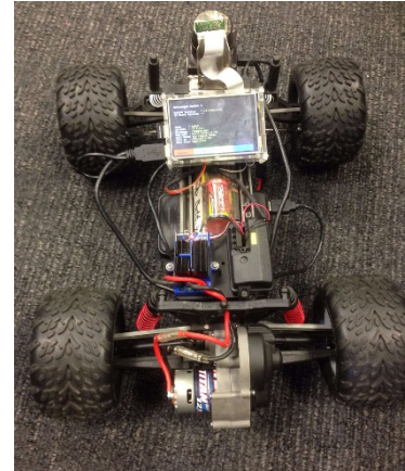
Figure 7.1: Model car with embedded controller, camera and Lidar
