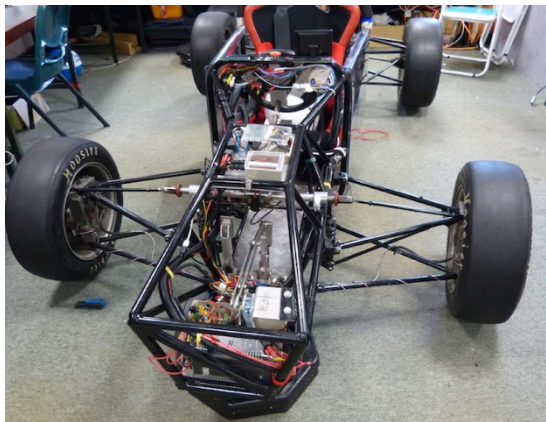
Figure 14.4: REV drive-by-wire control by Jordan Kalinowski
