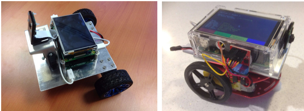
Figure 1.11: EyeCart robot (left with I/O controller) and simple robot chassis (right without I/O)
