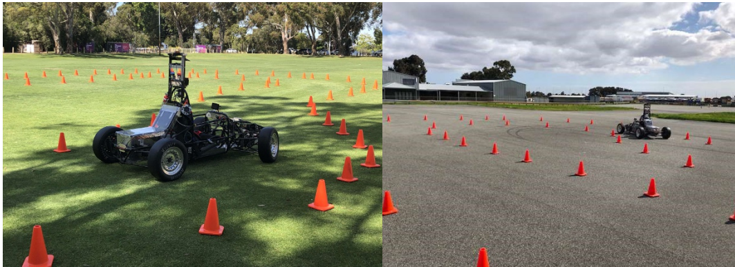
Figure 14.9: Autonomous cone-track driving on various test circuits
