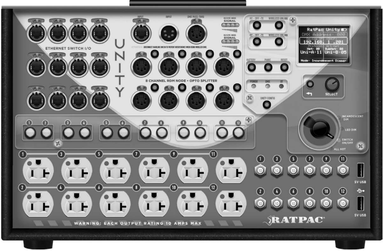
FIGURE 12.14 RatPac's Unity box is a combination Ethernet switch, Ethernet/DMX gateway, optical splitter, CRMX wireless transceiver (two), dimmer pack, and gang box.
