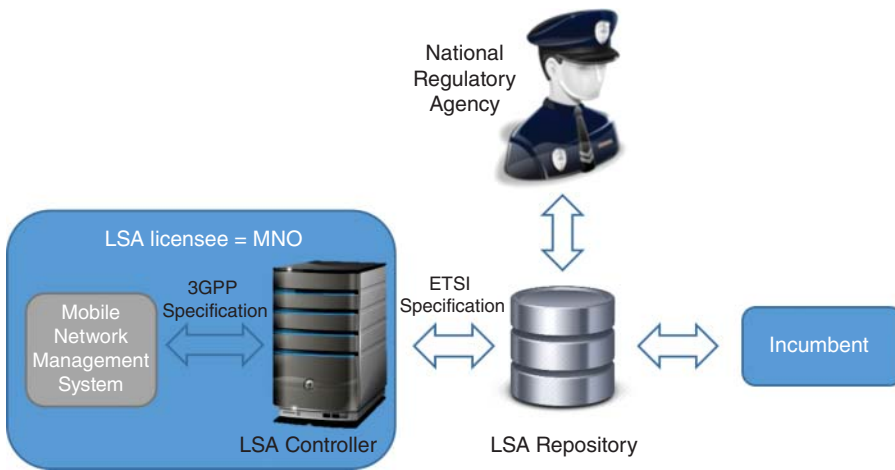
Figure 6.4 Architecture of a baseline LSA/ASA system operating at 2300–2400 MHz.
