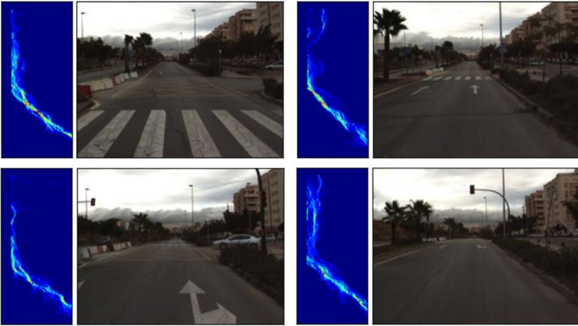
**FIGURE 8.6** Examples of four scenes with no obstacles: (right) the input image; (left) its corresponding V-disparity map.
