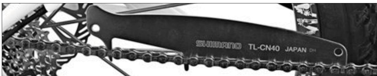
Using a chain checker, like one of the examples pictured above, allows you to gauge the wear of your chain. Replacing your chain at the correct time minimizes wear on expensive chainrings and cogsets.
