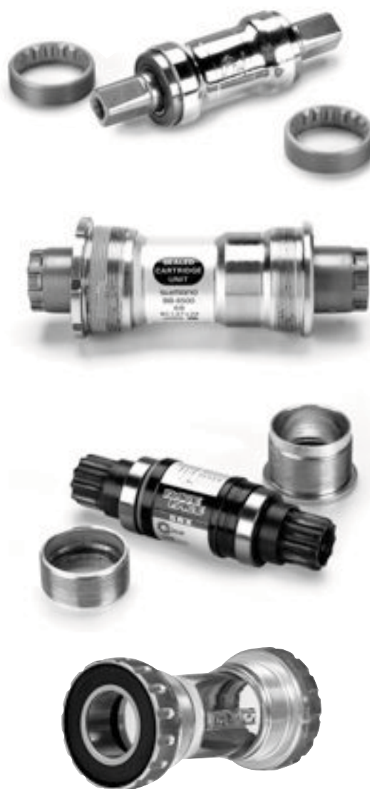
Bottom brackets come in several different configurations: square-taper (top), spline-fit (middle two), and external or two-piece (bottom). When replacing crankarms or bottom brackets, be sure which system you're using.
