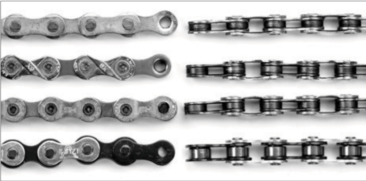
Close inspection reveals subtle differences in the shapes of different bicycle chains. Bulging and flared side plates help make derailleur chains (top 3 pairs) shift quickly and quietly, while the straight sides and broad rollers of track chains (bottom) give (bottom pair) them strength and help them stay on the chainring and cog where they belong.
