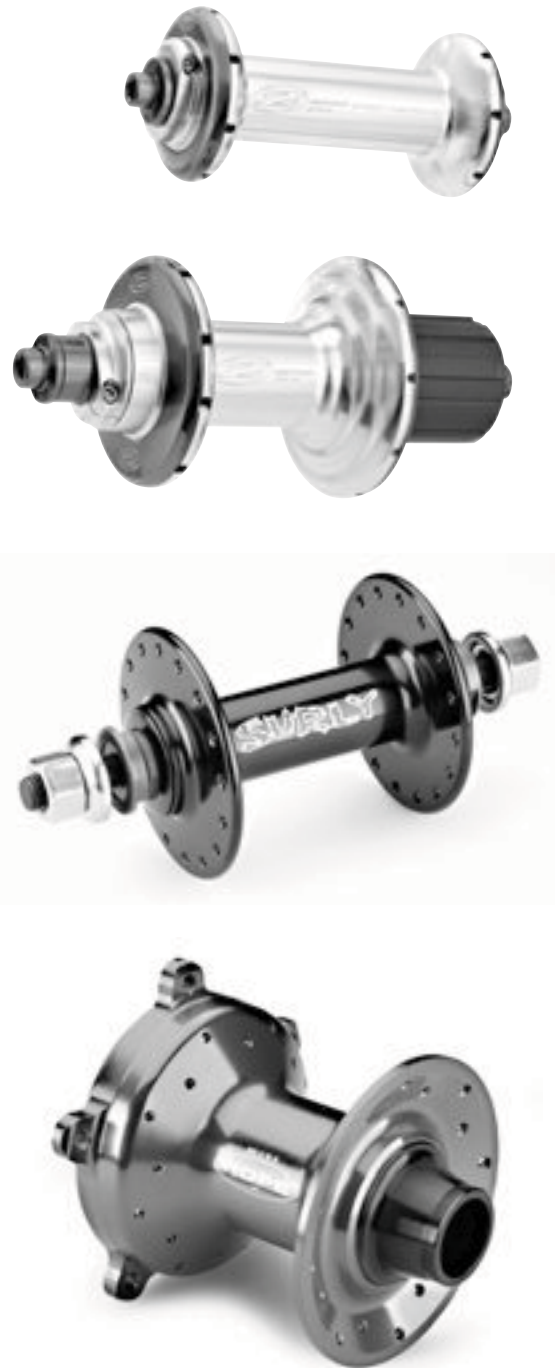
Axles can be held in place in several ways. Most common on modern bicycles are quick-release (QR) axles that use a cam-action skewer to grip the frame or fork dropouts on the axle (top). Solid axles use nuts to achieve this goal (middle), while through-axles (bottom) have a large-diameter axle that is clamped in place on specially designed frames and forks.
