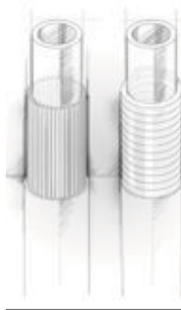
Spiral-wound cable housing (right) is strong and flexible, but it compresses slightly as the cable inside is pulled taut. The precision involved in modern 9-, 10-, and 11-speed indexed drivetrains makes linear or compressionless cable housing (left) necessary for accurate gear changes.
