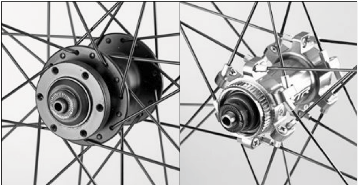
The Six-Bolt International Standard (left) is the most commonly found pattern for attaching brake discs. Shimano's CenterLock design (right) allows the use of a steel brake disc mounted on a splined alloy carrier to reduce weight and aid in heat dissipation.
