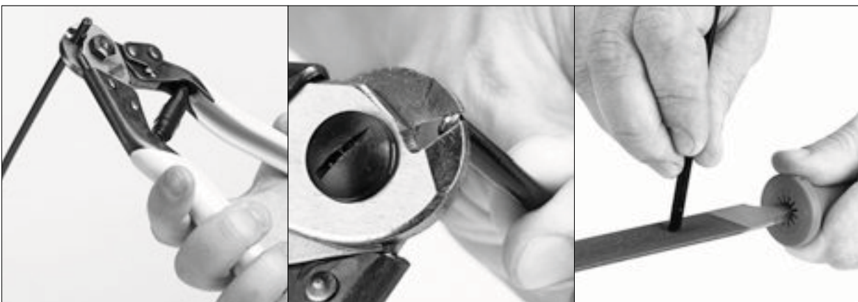
Cut cable housing using a sharp pair of cable or diagonal cutters. If a burr forms at the end, snip it away. File the end of the housing flat so it doesn't try to bite-in under pressure and bind the cable.
