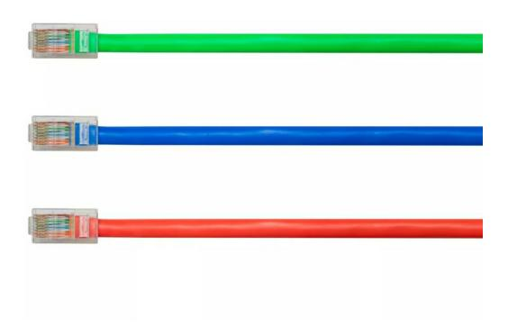
Telephone and data wiring are low-voltage wires used for "landline" telephones and internet hookups. Telephone cable may contain four or eight wires. Category 5 (Cat 5) cable, the most common type of household data wiring, contains eight wires wrapped together in four pairs. It can be used for both phone and data transmission and offers greater capacity and quality than standard phone wire.
