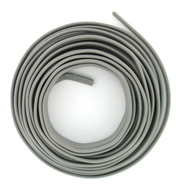
Underground Feeder (UF) is a type of nonmetallic cable designed for wet locations and direct burial in the ground. It is commonly used for supplying outdoor fixtures, such as lampposts. Like standard NM cable, UF contains insulated hot and neutral wires, plus a bare ground wire. But while sheathing on NM cable is a separate plastic wrap, UF cable sheathing is solid plastic that surrounds each wire. UF cable is normally sold with gray outer sheathing.
