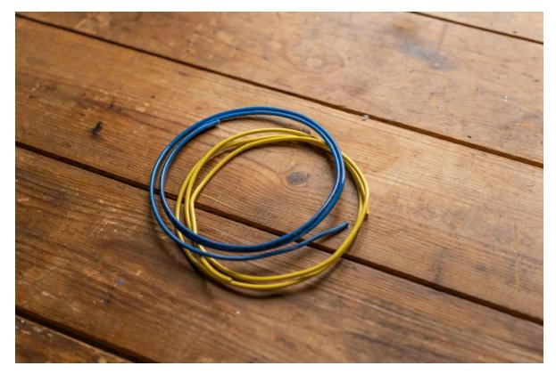
Rarely are blue and yellow wires found in NM cable. Blue wires are commonly used for travelers in a three-way and four-way switch applications.
