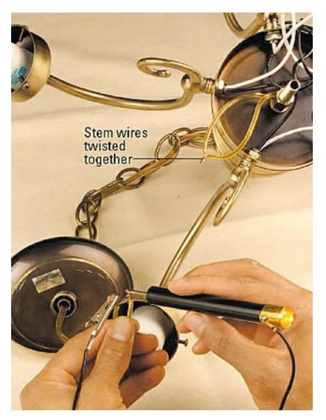
Disconnect the wires in the box, remove the chandelier, and place it on a work surface. Open the chandelier's junction box and pull out the wires. Test both the neutral (ribbed) and hot (smooth) wires for continuity.
