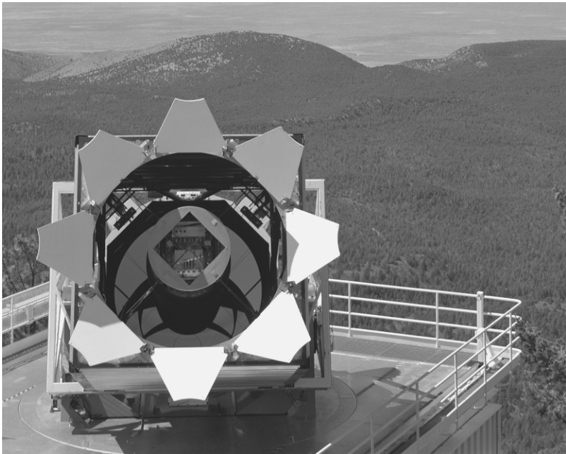
Figure 4 The Sloan Digital Sky Survey telescope in New Mexico. The main mirror is 2.4 metres across.
