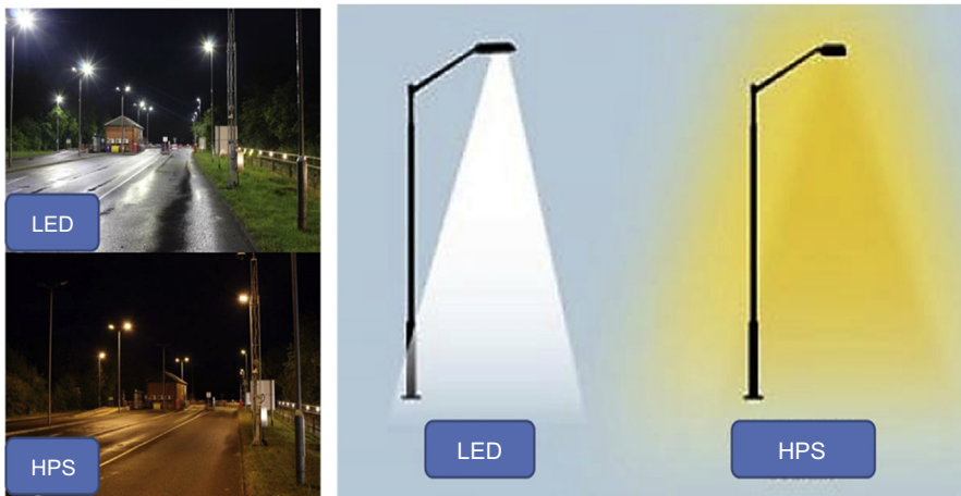
Figure 6.6 Comparison between the LED and the HPS street lights. HPS , high-pressure sodium; LED , light-emitting diode.
