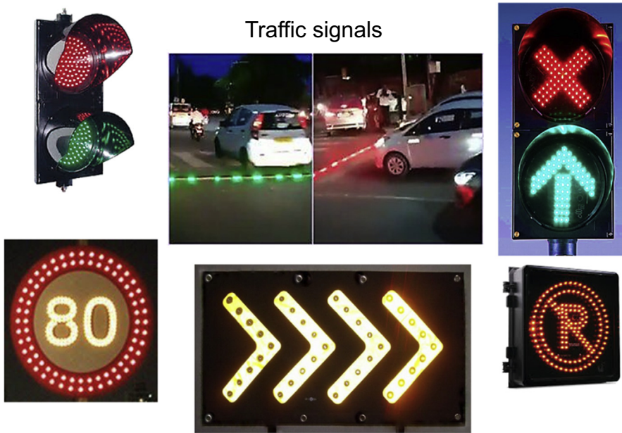
Figure 6.7 LEDs being used for traffic signal lights and signboards. LED , light-emitting diode.
