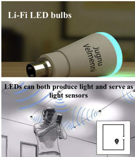
Figure 7.4 Li-Fi-compatible LED bulbs serving as transmitters and receivers for data transmission. LED , light-emitting diode; Li-Fi , liquid fidelity.
