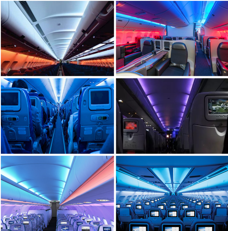
Figure 10.4 Color tunable aircraft cabin-lighting.
