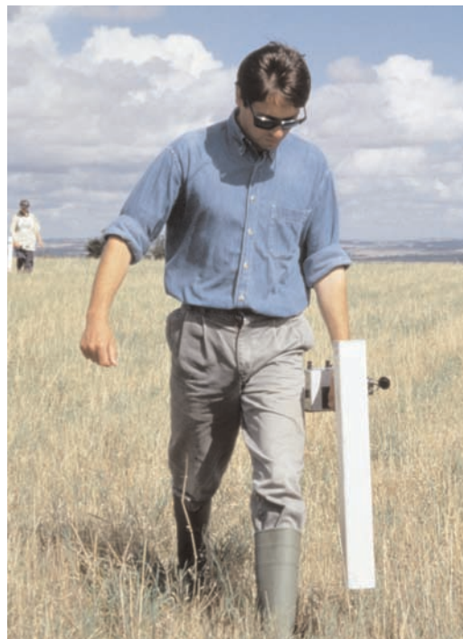
Fig 1.18 Magnetometer survey in progress using a Geoscan FM36 Fluxgate Gradiometer (from Archaeometry Branch, EH, Centre for Archaeology).
