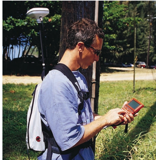
Fig 1.20 GPS surveying equipment used to produce the three dimensional topographical models of selected hillforts. a) Trimble Navigation 4600LS post-processing GPS equipment b) Leica Geosystems System 530 real-time kinematic equipment (from EH, Centre for Archaeology and courtesy of Leica Geosystems Ltd).
