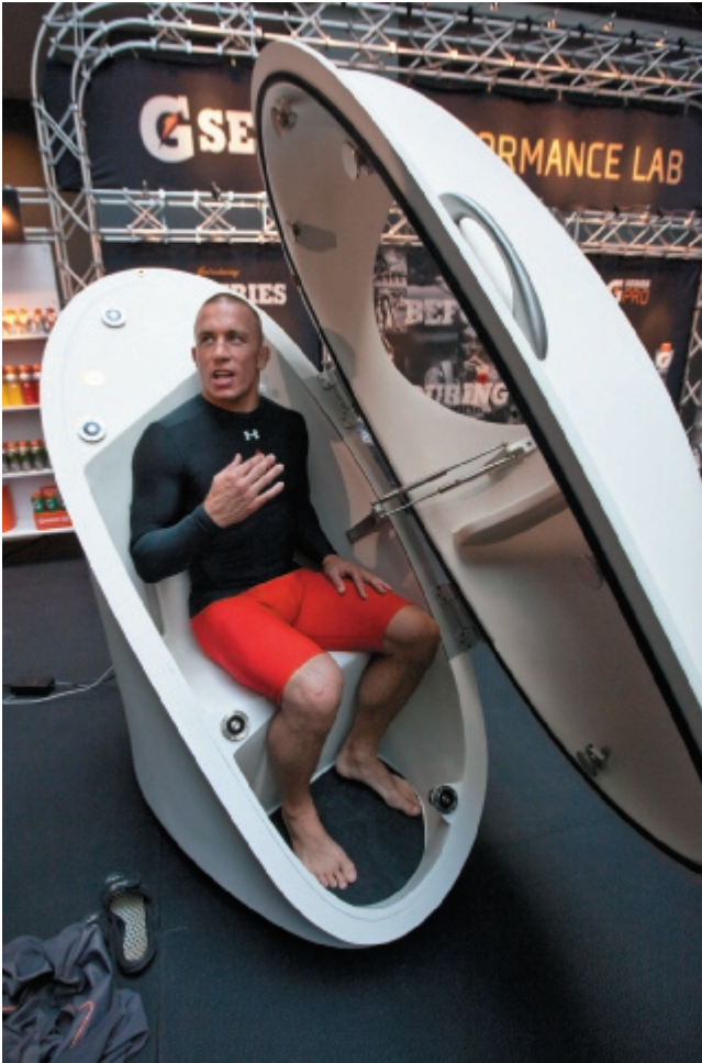
The Bod Pod® uses air displacement to measure body composition.
