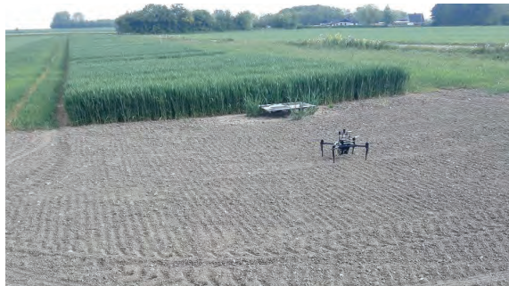
Figure 1. unmanned aerial vehicle (UAV) and experimental field on the day of data recording. A Matrice 100 UAV platform from DJI [32] was used.
