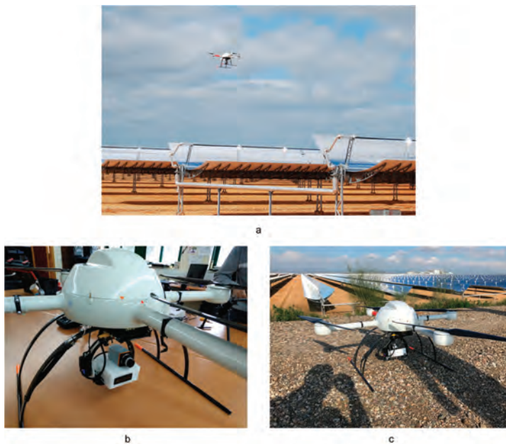
Figure 6. (a) The UAV performing an inspection on a concentrated solar power (CSP) plant; (b) Front view of the system onboard the UAV; (c) Back view of the system onboard.
