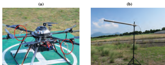
Figure 4. (a) antennas on the UAV marked as red circles; (b) the Yagi antenna at a ground station.
