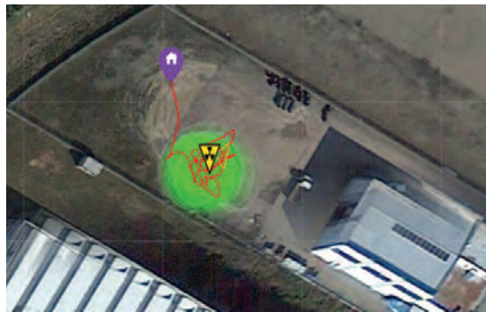
Figure 11. Detection of ^{192}\text{Ir} in the real environment (the operator has direct sight of the nuclear source): flight path of the experiment shown in Figure 10; regions where radiation was measured by the CdZnTe detector (green circles with different sizes and shading) and the estimated location of the maximum radiation (apex of the yellow triangle).
