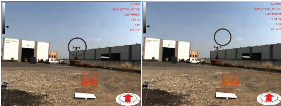
Figure 16. Comparison of UAV position estimation methods: vision-based (left), EKF (onboard sensors) (right). A video of the experiment is available as Supplementary Material (video2).
