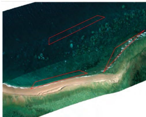
Figure 5. Multi-orthorectification by Headwall SpectralView overlaid in Google Earth, polygonal regions (in red) indicate visible spume regions in close proximity to coral.
