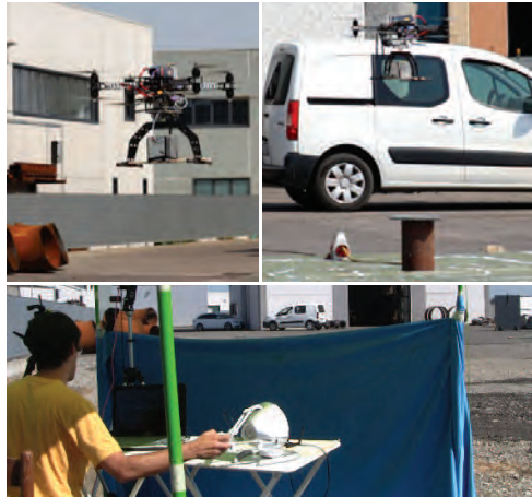
Figure 1. UAV equipped with a CdZnTe gamma-ray detector in flying tests (top). The operator using the visuo-haptic user interface (bottom). The operator sits in front of a cloth that prevents him from seeing the nuclear source on the ground.
