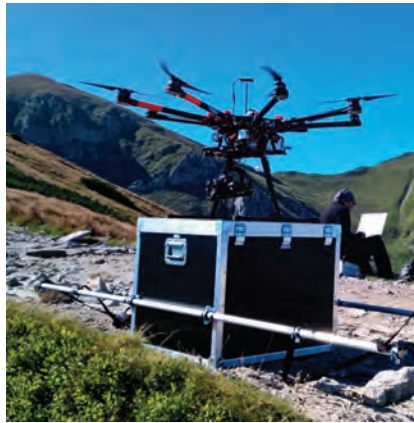
Figure 3. The device used for measurements, the DJI S1000 multicopter (source: authors' own study).
