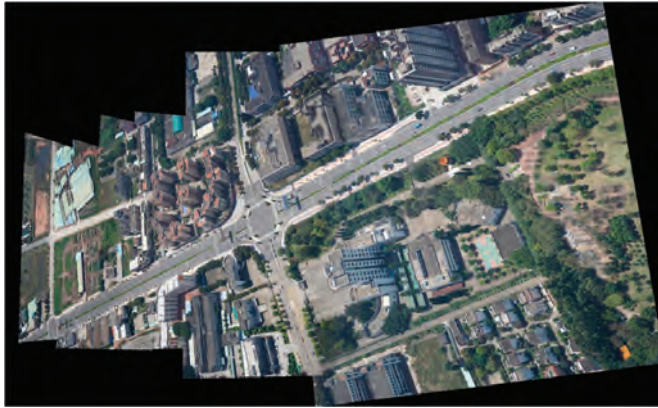
Figure 12. The stitching result of a single-strip image sequence.
