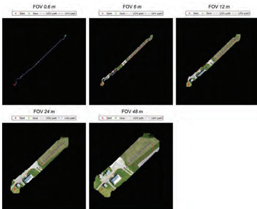
Figure 8. Paths corresponding to cases presented in Table 1. As the field of view of the simulated camera is expanded, the path cost is reduced despite an increase in distance traveled.
