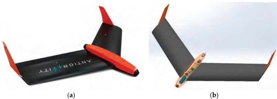
Figure 8. Research UAV: (a) Manufactured UAV; (b) UAV prototype in “Solidworks”.
