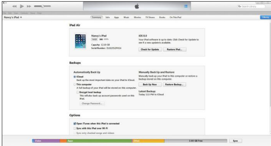
Figure 2-14: Go to the Summary tab to find out whether you need to update iOS.
