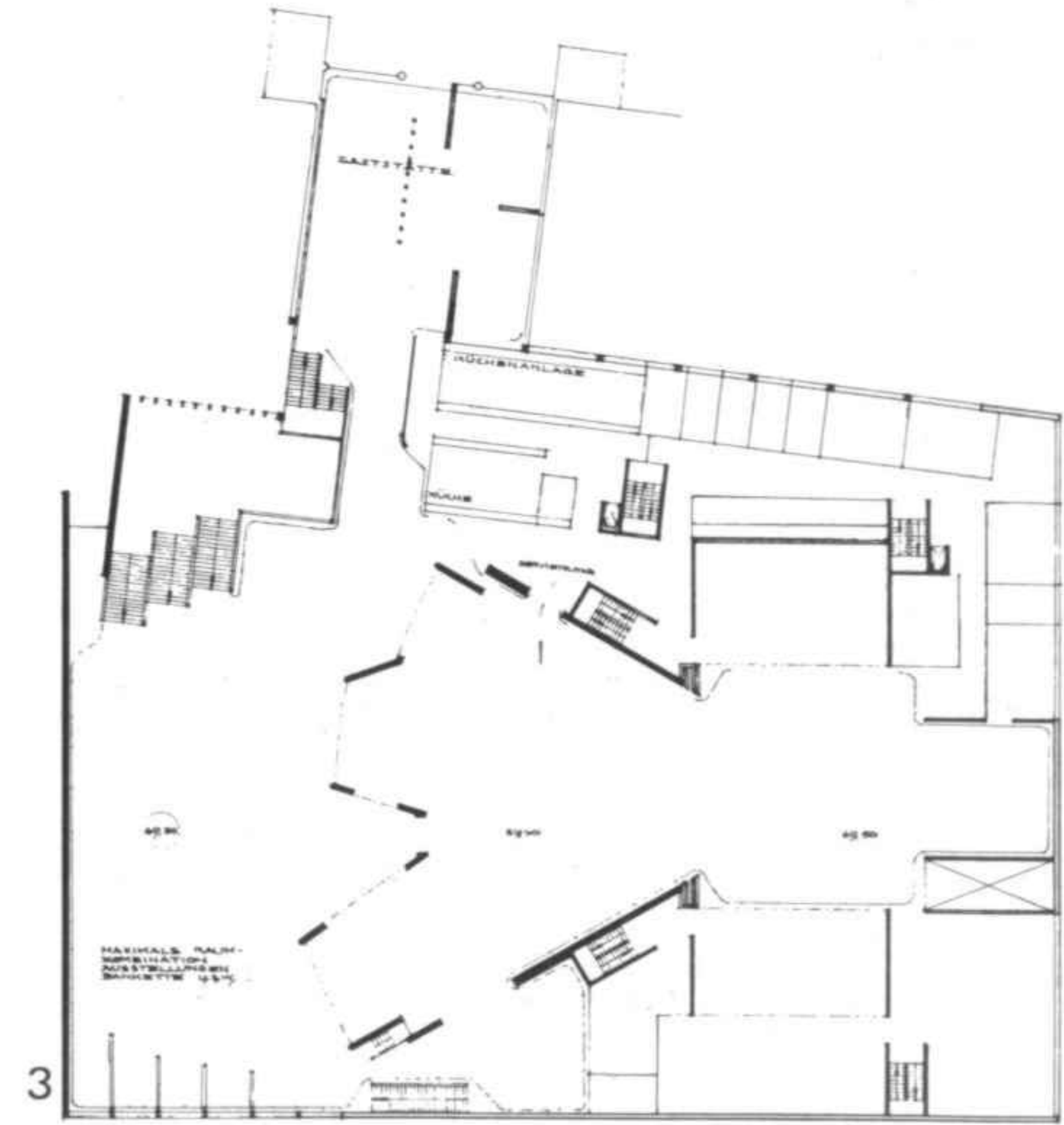
1 Large auditorium with panelling in place 2 Variant adapted for exhibitions with a small lecture theatre 3 The plan and sections show the variety of possible uses. The auditorium and stage are made up of a number of regular panels which can be set up or taken down 4 West facade as seen from the road; to the right, the auditorium 5 South facade
