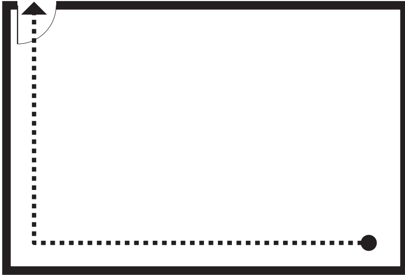
FIGURE 10.2.1-4. Acceptable travel distance path.
