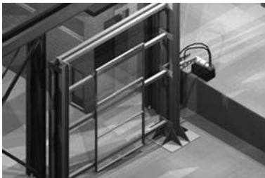
9.9 Schematic rendering of the AAMA 501.6 racking test facility.
