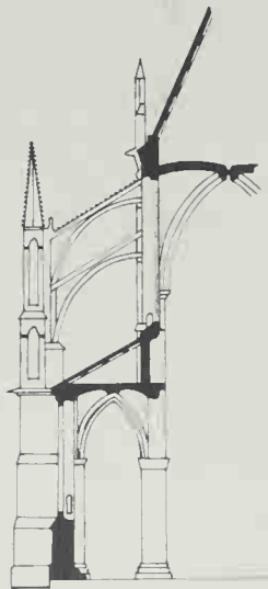
The Gothic masonry frame (Reims) avoids the lintel, a form in which the weight of stone makes it relatively weak; thus the vertical emphasis is a structural necessity.
