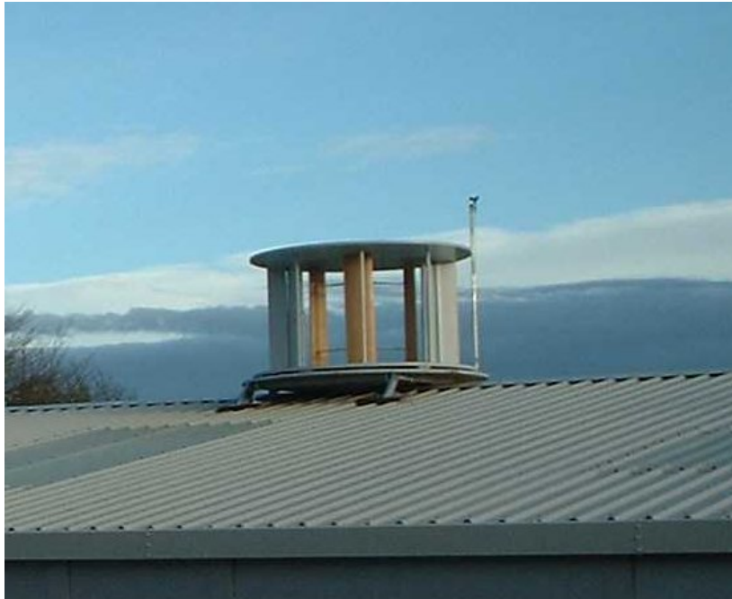
Figure 2-15: The Wind Dam VAWT prototype under test in November 2003.
