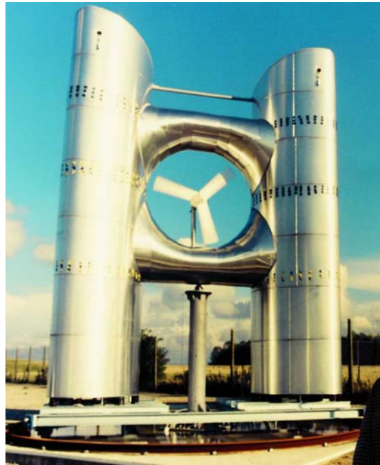
Figure 2-11: Photograph of the prototype WEB Concentrator during field-testing at CCLRC Rutherford Appleton Laboratory's Energy Research Unit Test Site.
