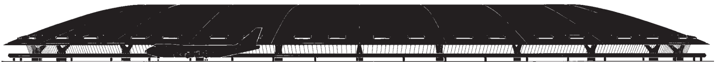
15.19 Elevation of Grimshaw's design for Terminal 5. The concept owes something to Andreu's circular forms employed at Charles de Gaulle Airport, though here modified by the need for natural ventilation.
