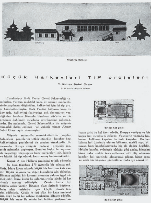
FIGURE 6.12. SMALL-TYPE HALKEVI BUILDING TEMPLATE PROPOSED BY THE ARCHITECTURE OFFICE OF THE REPUBLICAN PEOPLE'S PARTY. NOTE THAT THE PLAN FEATURES AN AUDITORIUM THAT IS LARGER IN COMPARISON WITH SPACES FOR OTHER FUNCTIONS OFFERED BY THE FACILITY, THUS EMPHASIZING ITS DIDACTIC FUNCTION. COURTESY OF THE LIBRARY OF THE CHAMBER OF ARCHITECTS OF TURKEY.
