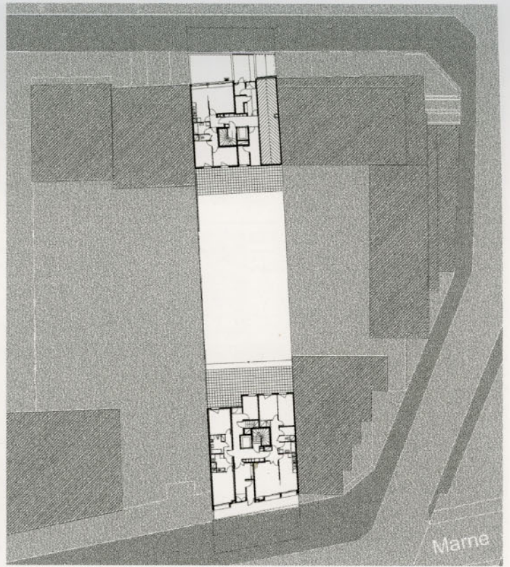
The narrow lot, measuring 13 by 68 meters, inspired the arrangement of two blocks and a spacious central garden courtyard. The double block visually distances itself from the traditional social housing image via large openings facing the canal.
